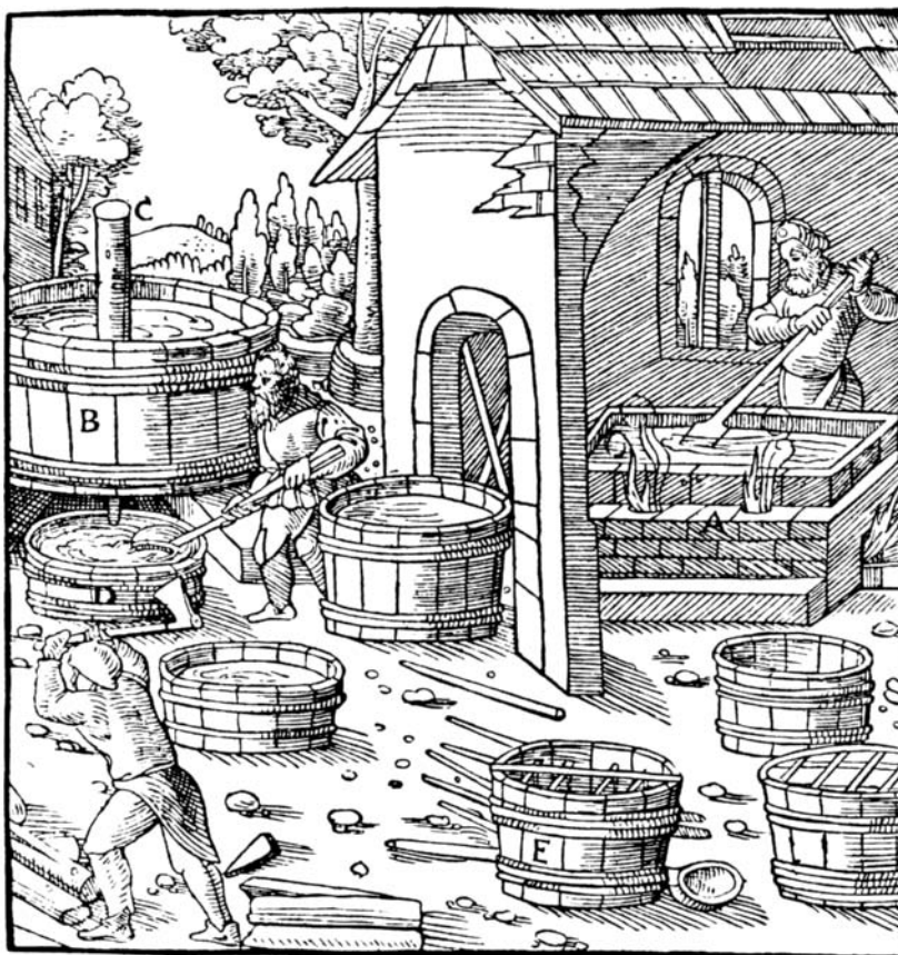
Figure 74.1 Saltpeter production in the Middle Ages. Soil saltpeter is leached with water in a tub (B) that contains a layer of sand in the bottom and a plug (C). Filtrate is collected in another tub (D) and is reduced in a copper vat (A), which is heated over a hearth. Reduced solution is placed in crystallization containers (E) where saltpeter crystallizes on copper sticks. From De Re Metallica (On the Nature of Metals) by Georgius Agricola (1494–1555), published in 1556.
