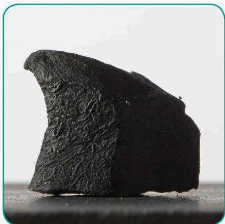
1. This piece of pure lithium is placed on a surface and is exposed to the air.
