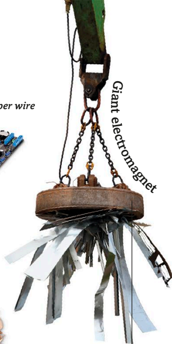
Massive crane-mounted electromagnets contain huge coils of copper wire.
