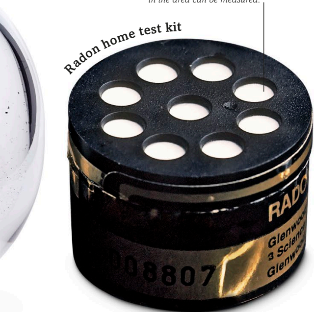
This kit collects radon from the air so the amount of the gas in the area can be measured.
