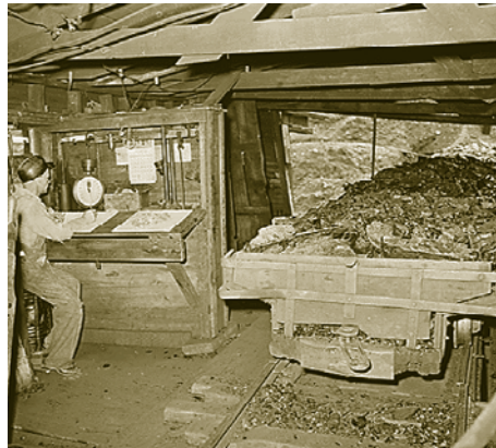
tipple At a Harlan County, Kentucky mine, a worker checks the weight of coal moving from the tipple to railway freight cars.
