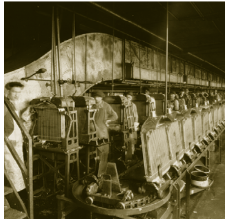
assembly line Workers on a radiator soldering line at a Ford assembly plant, 1923.
