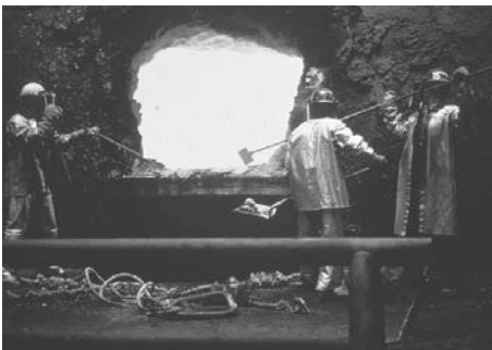
furnace A contemporary blast furnace used for steelmaking; its temperatures can reach 1650°C (3000°F).
