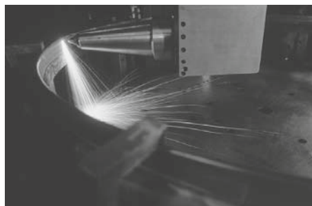
laser Laser beam employed in the process of manufacturing a jet engine part.
