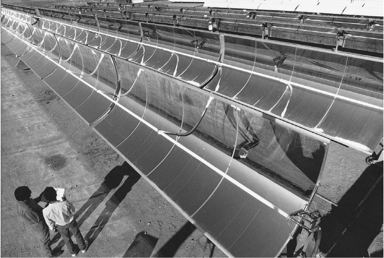
Researchers at Sandia National Labs use a trough of parabolic mirrors to focus sunlight on a long glass tube in order to detoxify water. (U.S. Department of Energy)
