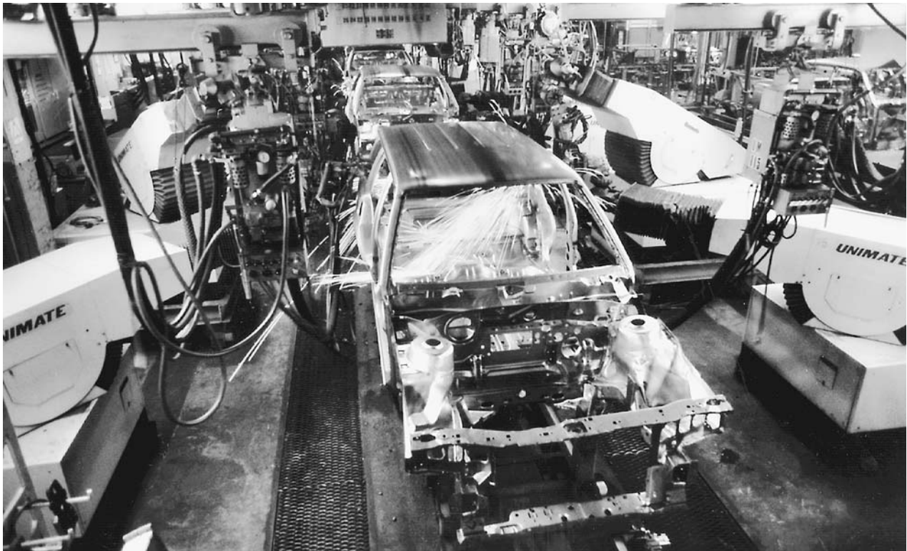
Automobile assembly line with welding robots. The automobile industry relies heavily on automation in many parts of its manufacturing process. (AP/Wide World Photos.)
