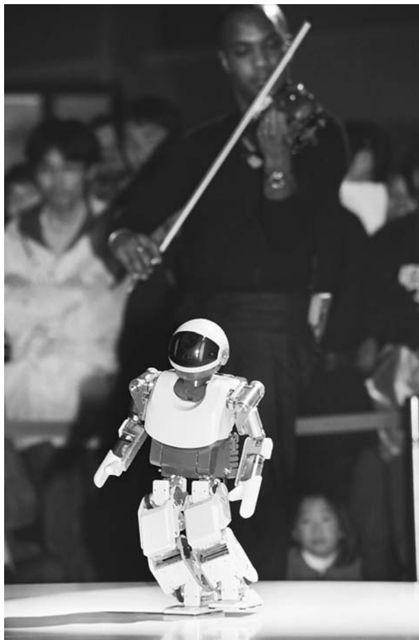
Android SDR-3X. Sensory cells beneath its “feet,” a camera, and a microphone enable it to walk, talk, and dance. (© Hashimoto Noboru/Corbis Sygma.)
