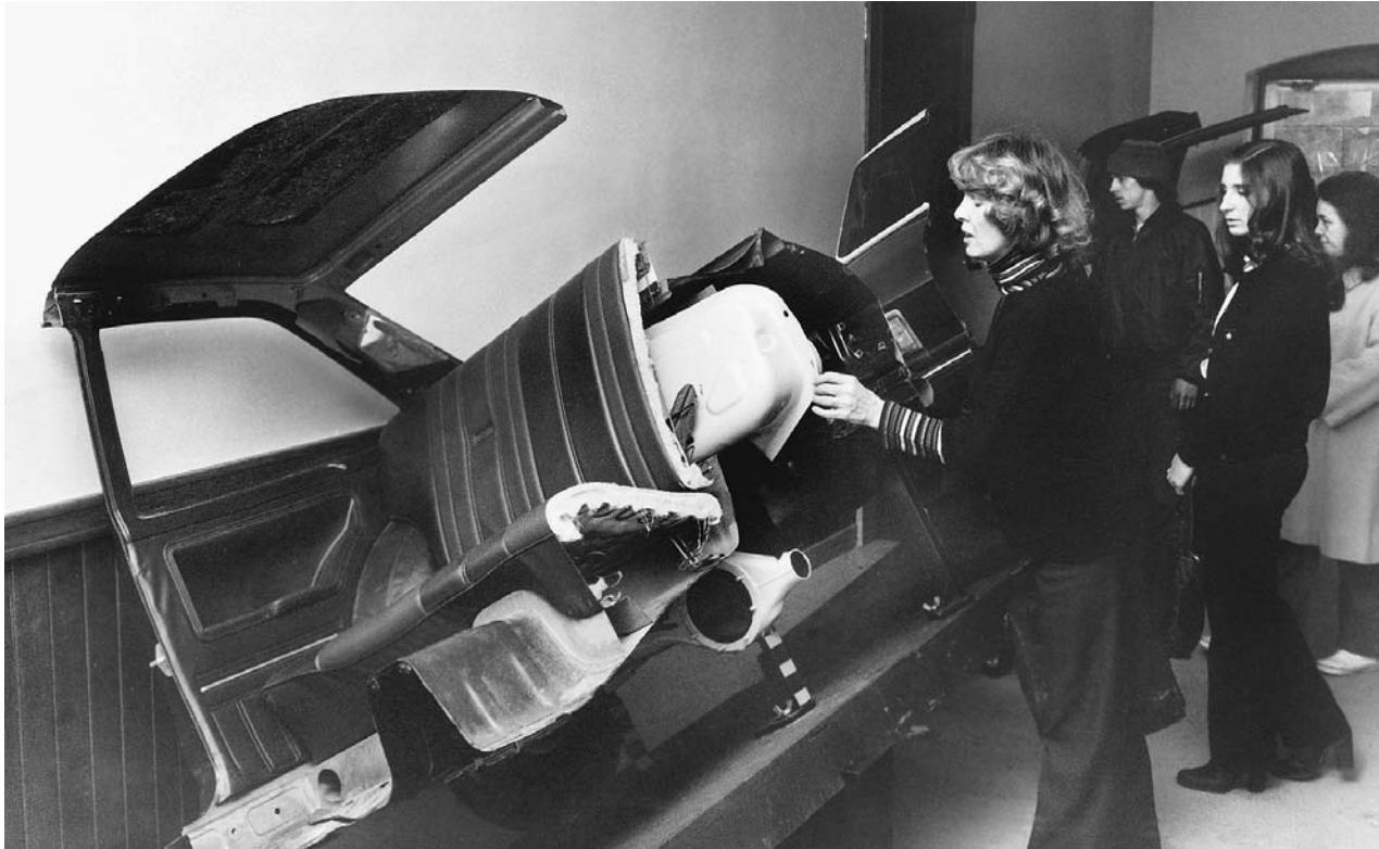
People examining close-ups of a Ford Pinto wagon in the basement of a courthouse. The wagon was used as evidence in a murder trial resulting from a fatal accident in which the gas tank exploded upon collision. ( Art Shay/Getty Images. )
