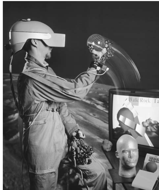
A man demonstrates a virtual reality device by lifting a virtual rock on a simulated Martian surface, wearing a video helmet and virtual reality gloves. (© Roger Ressmeyer/Corbis.)
