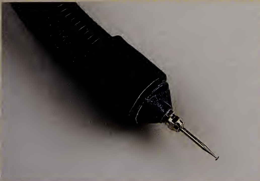
This turbine drill is designed to be attached to a vacuum cleaner. The cutting bit consists of a 3mm ( \frac{1}{8} in) disc
