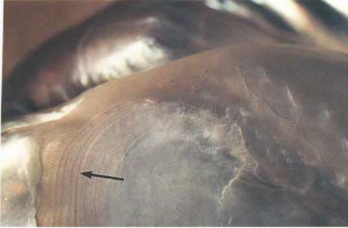
Fig. 6. Surface growth lines on the back of the Hope Pearl indicating its blister origin. 5x.
