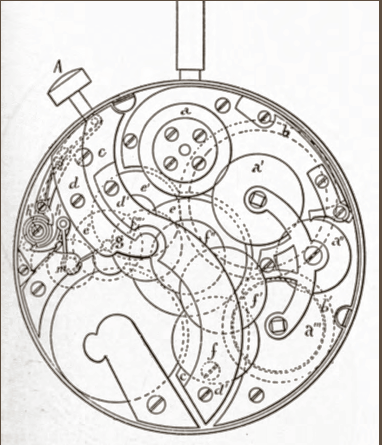
Adrien Philippe's independent dead seconds mechanism, Swiss patent number 1017 of 23 May 1889.
