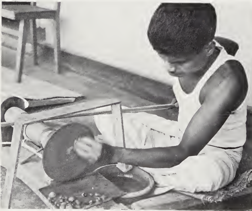
Below right Cleaving a diamond. The receptacle on the right receives the diamond dust from the previous operation of scratching a nick (kerf) into which the cleaving blade can be inserted.
