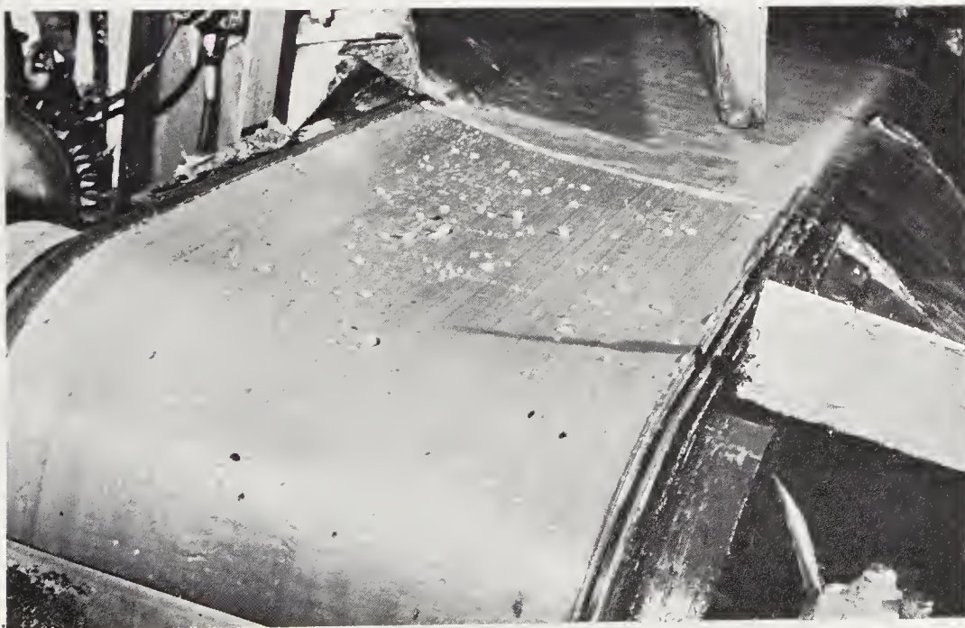
A grease belt separator. Diamonds stick to the grease while other stones are flushed away by the water.
