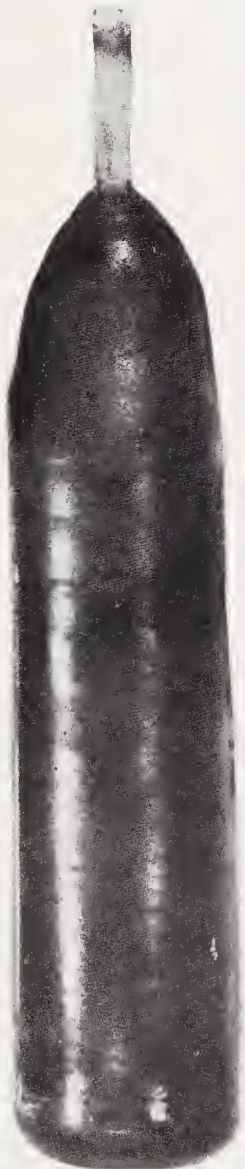
A modern boule of a synthetic corundum gemstone formed by the Verneuil flame fusion method.
