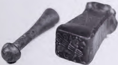
29 (below) Two ancient bronze punches used by goldsmiths. The Roman one (left) was for forming domes, the earlier Western Asiatic one (right) produced an animal design. Private collection.
