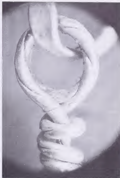
11 (right) Optical microscope view of a wire link from a Roman necklace, showing the spiral 'seam' characteristic of much ancient wire. About 20× magnification.
