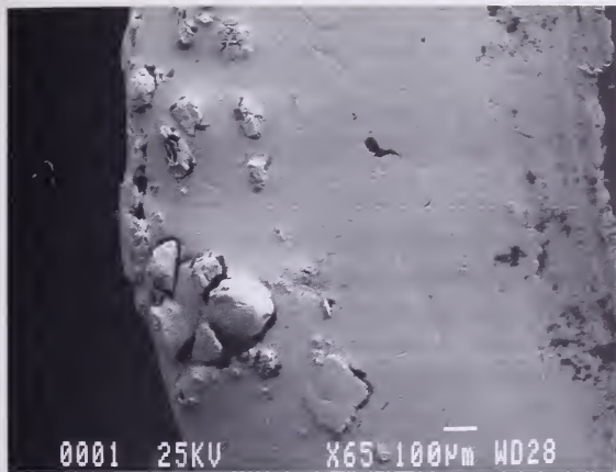
10 (above) Scanning electron microscope view of the platinum-metal inclusions visible on the surface of a Roman gold ring.
