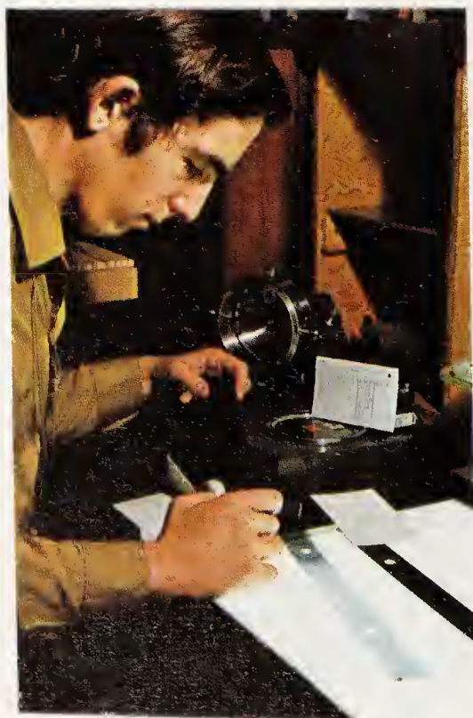
28 Electron microprobe X-ray analyzer (top) reveals chemical composition of minerals; X-ray powder cameras (above) identify them. Author measures X-ray powder photo (r.).
