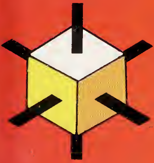
ISOMETRIC All axial angles are 90 degrees, all axes equal length.
