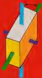
MONOCLINIC 1 axial angle variable, all axes different lengths.
