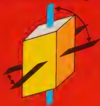
TRICLINIC All axial angles and axis lengths variable.
