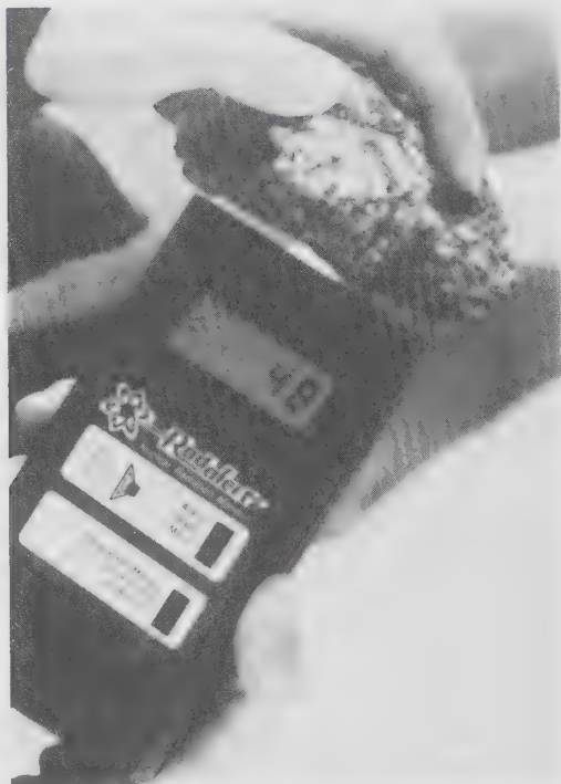
Modern miniaturized radiation monitors easily detect elevated radiation levels in radioactive minerals.
