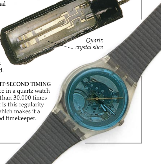
WATCH PIECE This microthin quartz crystal slice is used to keep time in a quartz watch. The photograph is greatly enlarged.
