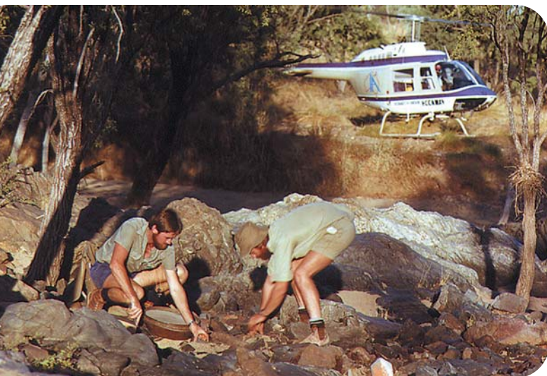
Figure 5. Two geologists sample stream gravels in a remote portion of the Kimberley region in Western Australia to locate diamond indicator minerals. The size of the region, and its remoteness, meant that a helicopter was needed to reach sites targeted for diamond exploration. Here, the geologists are excavating a heavy-mineral sample from gravel trapped behind a natural rock dam in a creek. A special geologic laboratory was set up in Perth to evaluate the mineral content of such samples.
