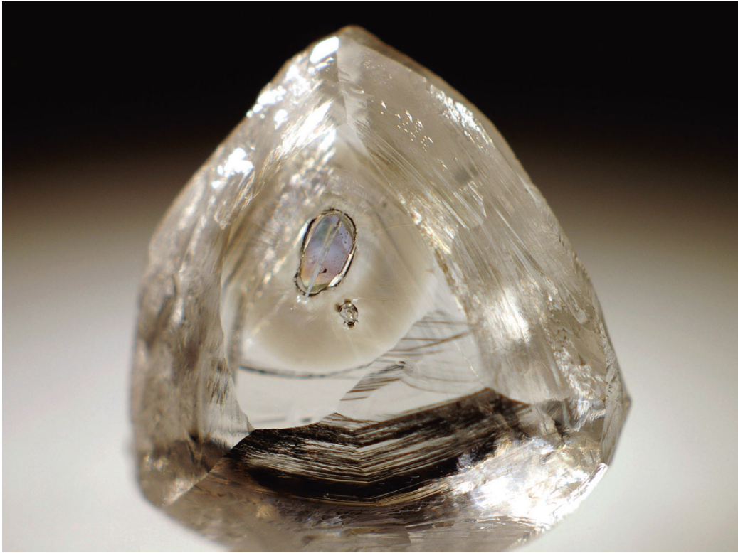
5-02: Left , Colorless inclusions (large inclusion is ~1 mm) of an unknown mineral in a flattened dodecahedral diamond from the Venetia mine, South Africa. The main crystal face of the large inclusion is oriented parallel to a relict octahedral crystal face of the diamond. The diamond has been polished for better visibility. Below left , Close-up of the inclusions. It is notable that the crystal faces of the smaller inclusion are oriented in the same direction as those of the larger inclusion.
