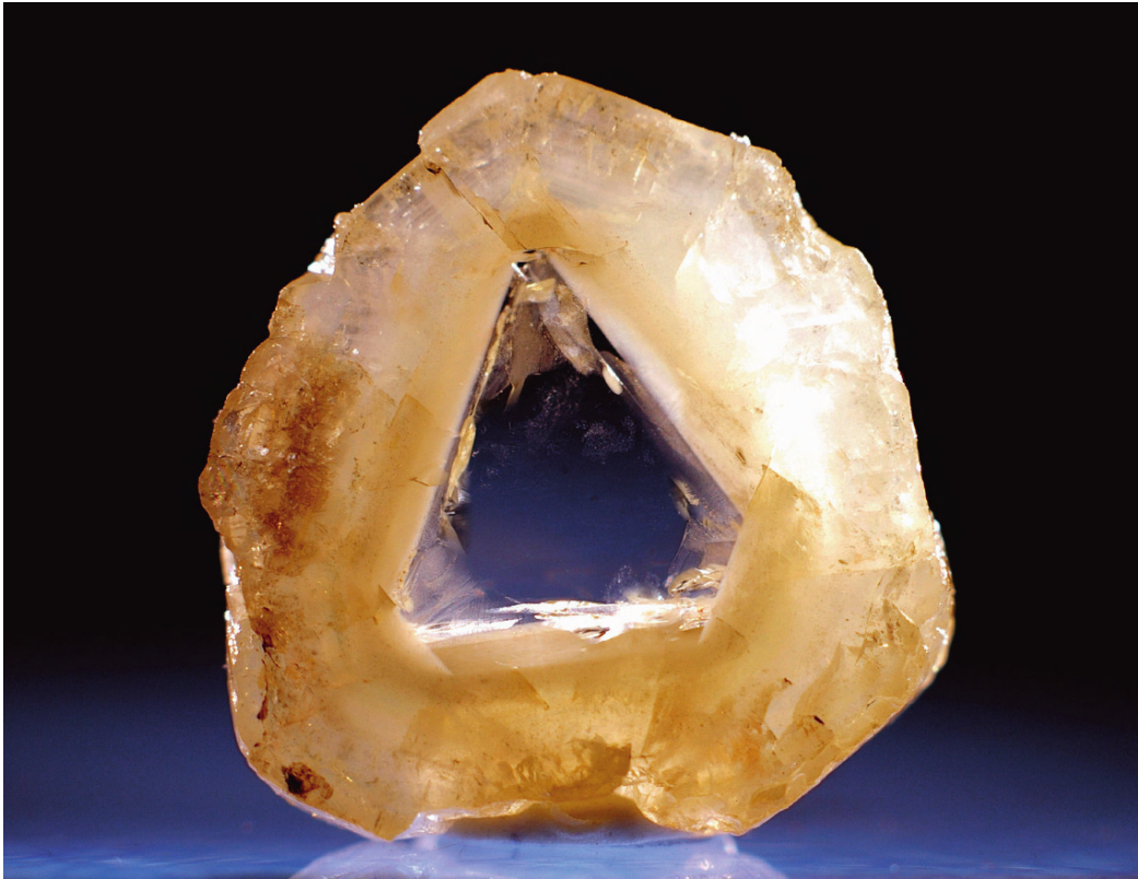
2-53: Polished section through a sharp-edged octahedral diamond with a thick fibrous coat ( \varnothing : ~7 mm). The fibrous coat exhibits faint concentric layering.
