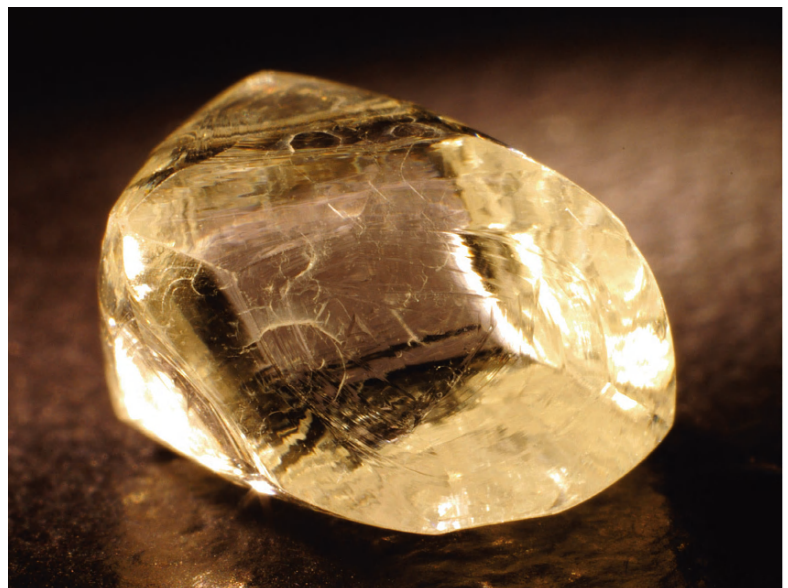
4-39: Pale yellow, dodecahedral diamond (1.11 ct) with large crescent-shaped percussion marks that formed as a result of particle impact during transport.
