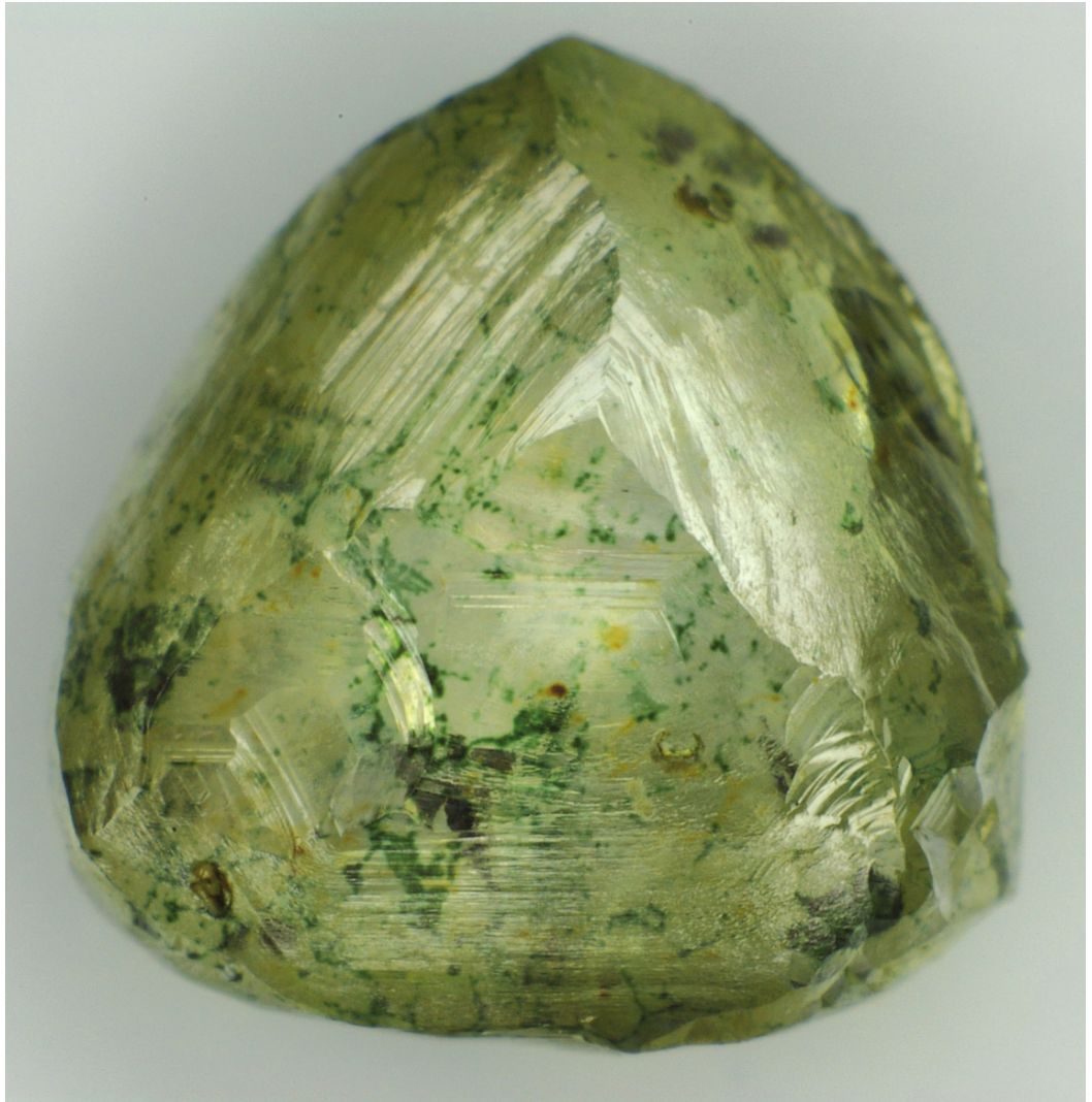
3-36: Dodecahedral macle from Brazil with numerous green surface spots and a few brown surface spots ( \varnothing : ~6 mm).
