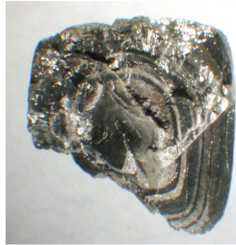
2-47: Fragment of a hailstone boart from Diavik, Northwest Territories, Canada ( \varnothing : ~8 mm). The concentric layers, which are exposed on a fracture plane, consist of fibrous (grey) and polycrystalline (white) diamond. The habit of the hailstone boart is cubic.
