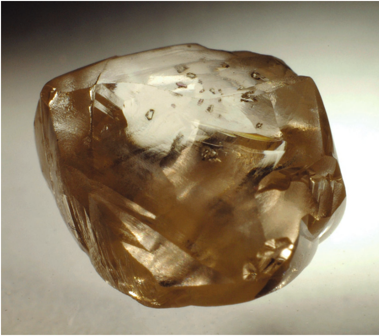
2-26: Irregular diamond with a smooth undulated surface and a light brown color (1.19 ct). The appearance of this diamond is typical for Type II diamonds. This diamond also contains several colorless mineral inclusions.
