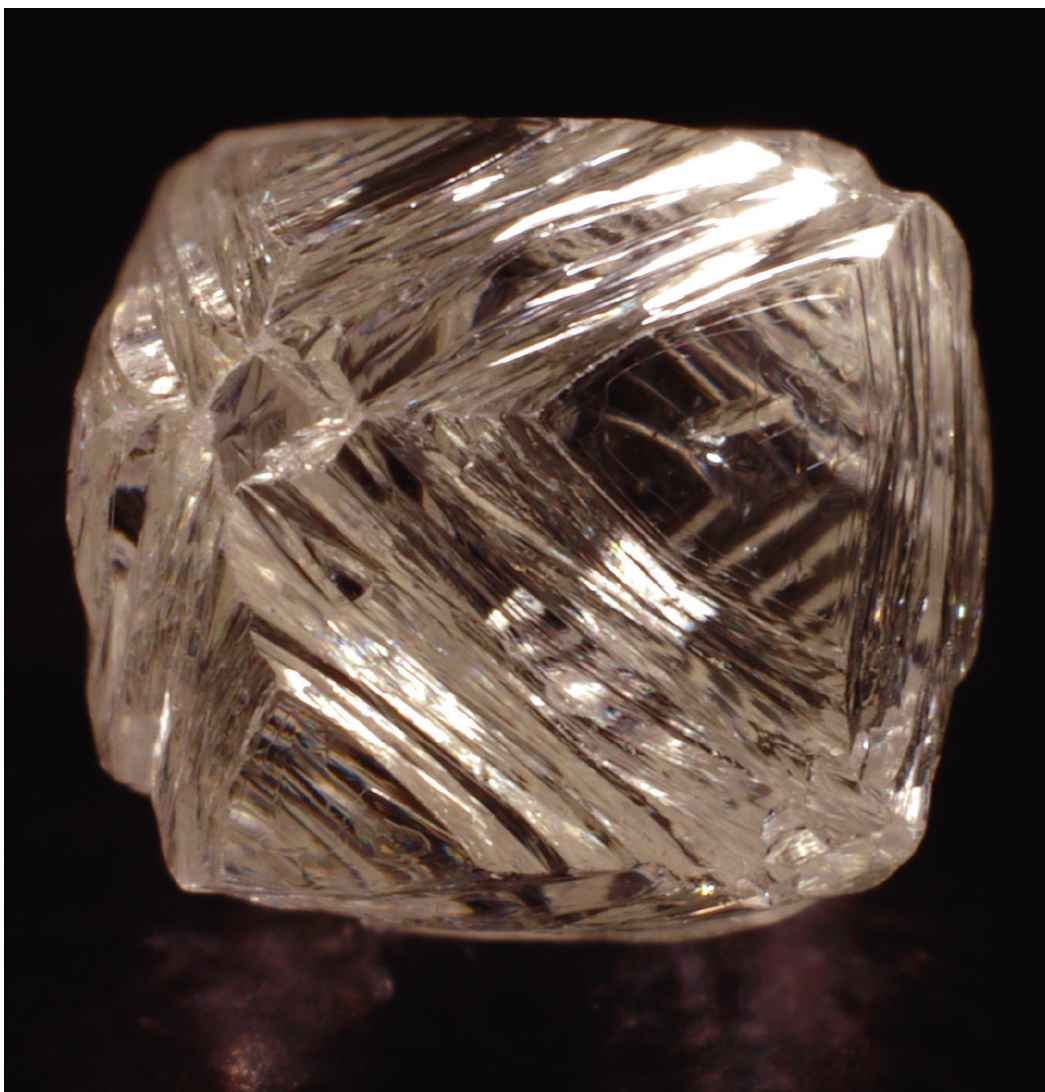
2-05: Stepped, octahedral diamond with slightly rounded crystal edges (0.96 ct).
