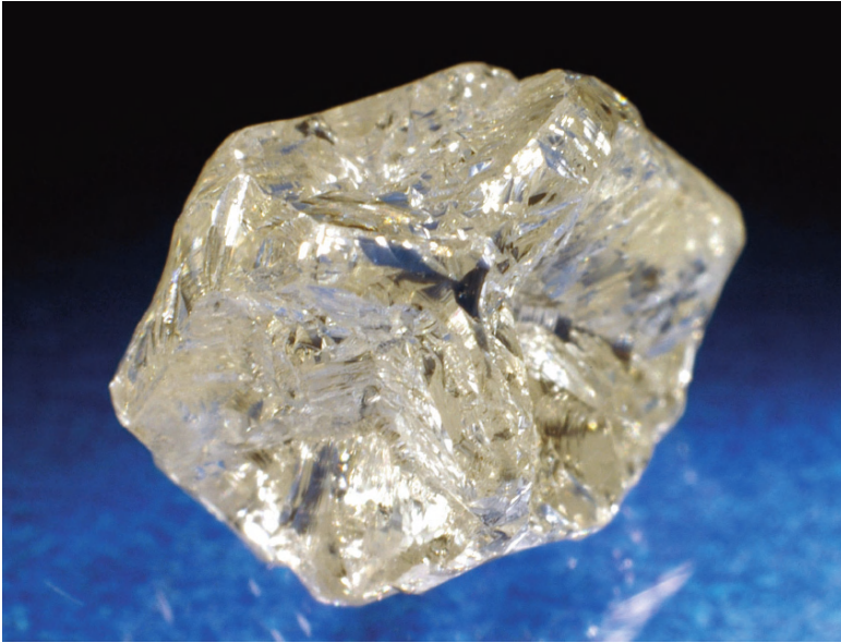
2-14: Left , Re-entrant diamond cube (1.19 ct). The strongly concave crystal faces result in a skeletal appearance. Above , Simplified representation of the crystal faces. Miller indices mark subordinate octahedral crystal faces.
