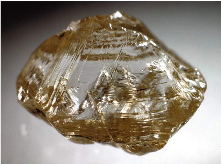
4-07: Light brown diamond with multiple imbricated shield-shaped laminae (1.11 ct).
