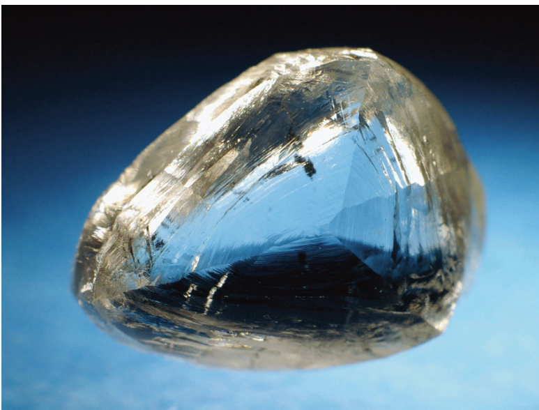
2-38: Strongly rounded and slightly distorted dodecahedral macle (1.13 ct).
