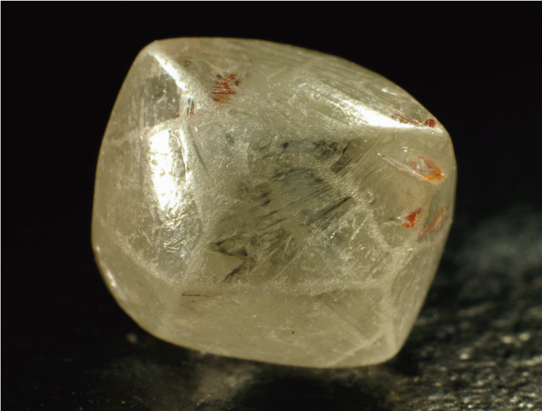
4-43: Dodecahedral diamond (1.13 ct) with abraded edges and scratched crystal faces. Inclusions inside the diamond cause the orange color.
