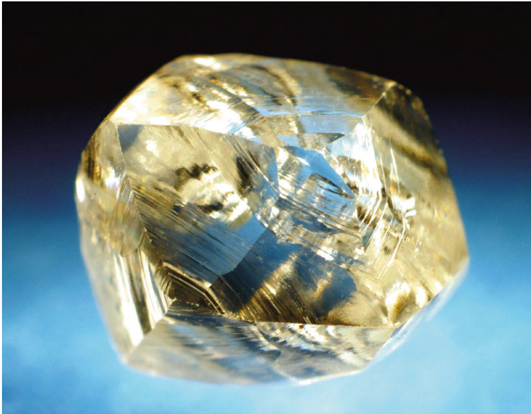
4-17: Left , Concentric terraces on the surface of a rounded dodecahedral diamond (1.00 ct). Below , Simplified representation of the main crystal faces with the terraces outlined in red.
