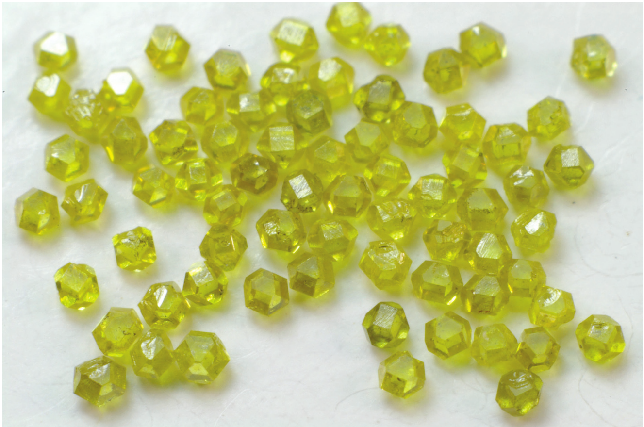
3-11: Synthetic diamonds with cubo-octahedral habit, exhibiting the characteristic yellow color of pure Type Ib diamonds, which is caused by single-substitutional nitrogen impurities. The nitrogen in synthetic diamonds is of atmospheric origin. The field of view is ~1.5 cm.
