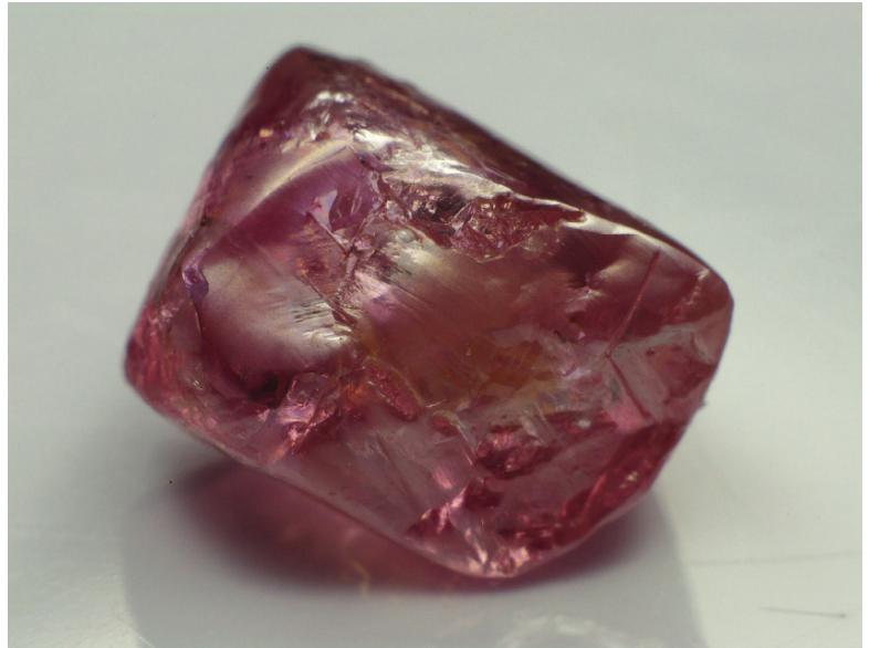
3-23: Pink dodecahedral diamond from the Bow River alluvial deposit, Western Australia (1.28 ct).
