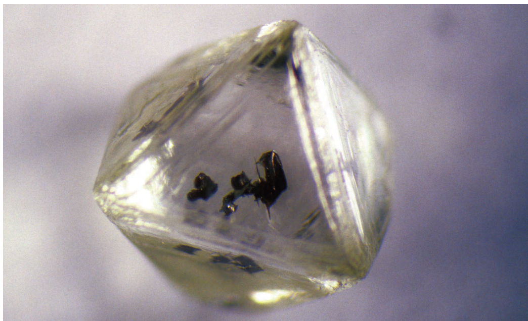
5-18: Smear-out sulfide material on fractures in a diamond ( \varnothing : ~3 mm) from the Jagersfontein mine, South Africa.
