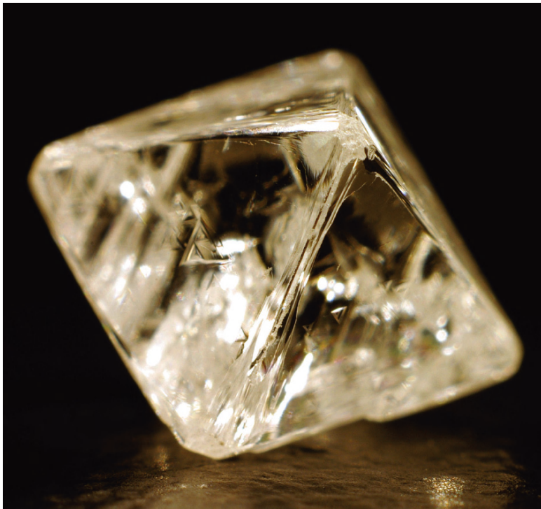
2-03: Diamond octahedron with minor resorption at the crystal edges (1.08 ct). The crystal faces exhibit several triangular etch pits (trigons).
