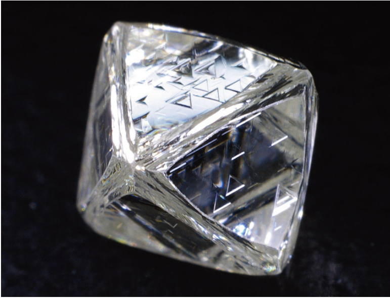
2-06: Octahedral diamond with resorbed crystal edges and corners (0.96 ct). Numerous triangular etch pits (trigons) indicate that the octahedral crystal faces were also affected by the resorption.
