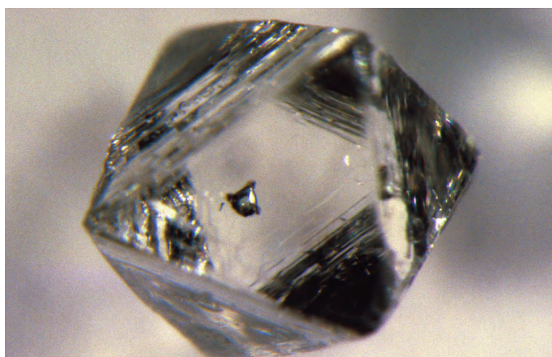
5-07: A colorless mineral inclusion in an octahedral diamond (0.04 ct) from the Jagersfontein mine, South Africa. After it was released from the host diamond, the inclusion was identified as an eclogitic clinopyroxene.
