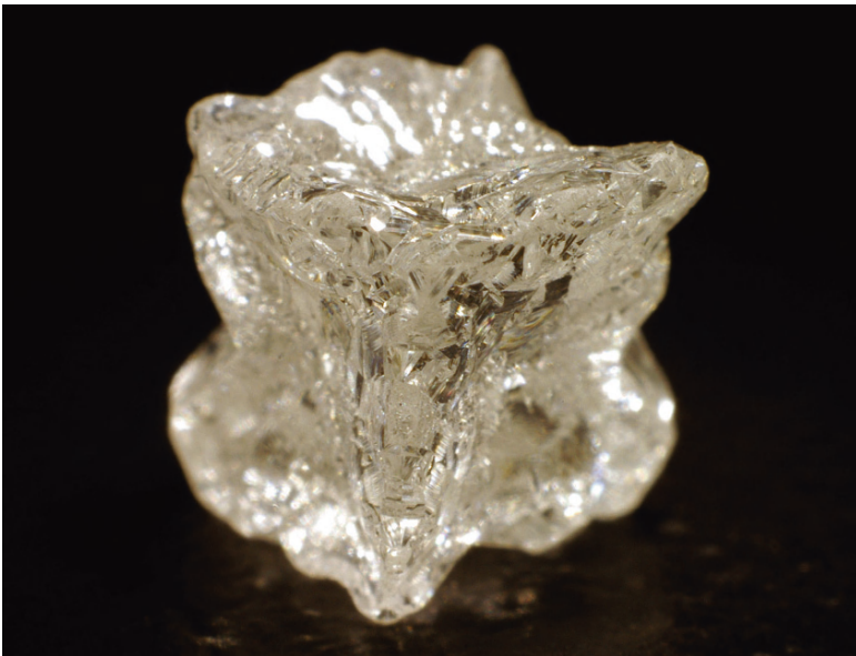
2-15: Left , Re-entrant diamond cube with re-entrant facets along the crystal edges (1.03 ct). Above , Simplified representation of the crystal faces. The re-entrant facets along the crystal edges are marked in grey.
