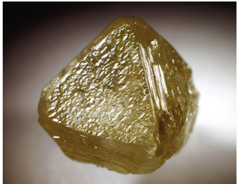
2-52: Octahedral diamond with a thin fibrous coat (1.19 ct). The octahedral crystal faces are marked by numerous trigons.
