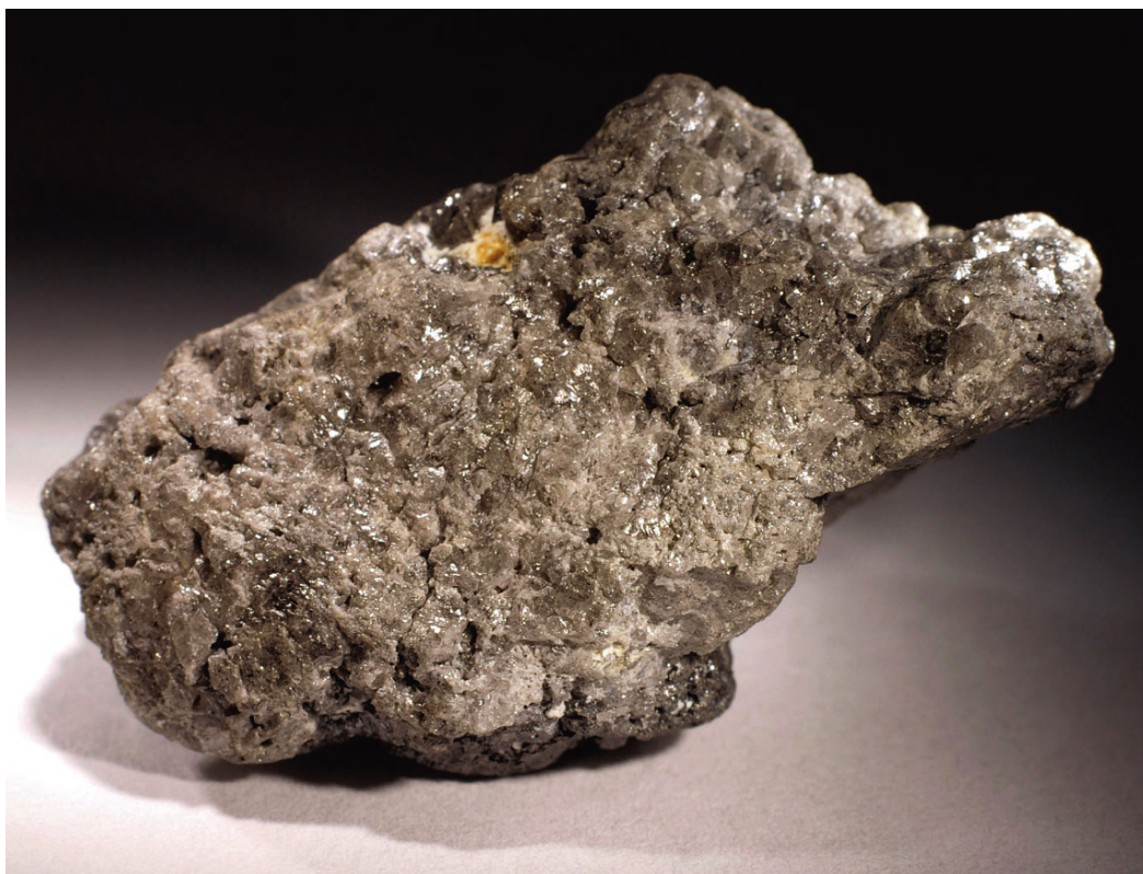
2-55: Framesite: a granular variety of polycrystalline diamond ( \varnothing : ~3 cm).
