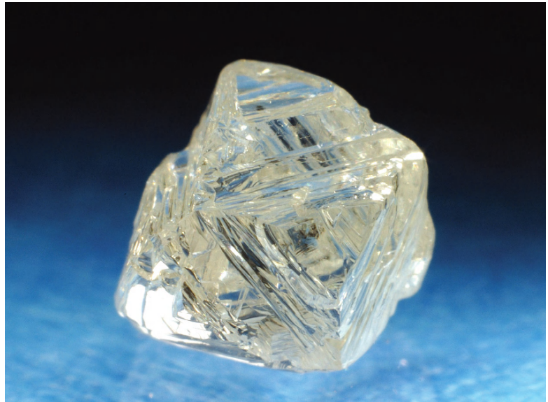
4-02: Octahedral diamond with multiple triangular growth plates of variable thickness (0.92 ct). The growth plates cause the stepped appearance of this diamond.
