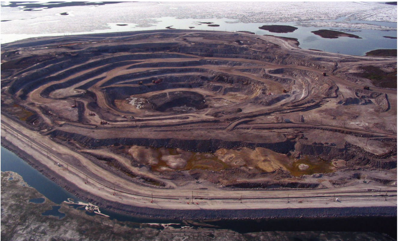
1-14: Aerial view of an open pit (A-154 kimberlite pipe) at the Diavik mine, Northwest Territories, Canada, in the early stages of development. The kimberlite is exposed in the central part of the pit.
