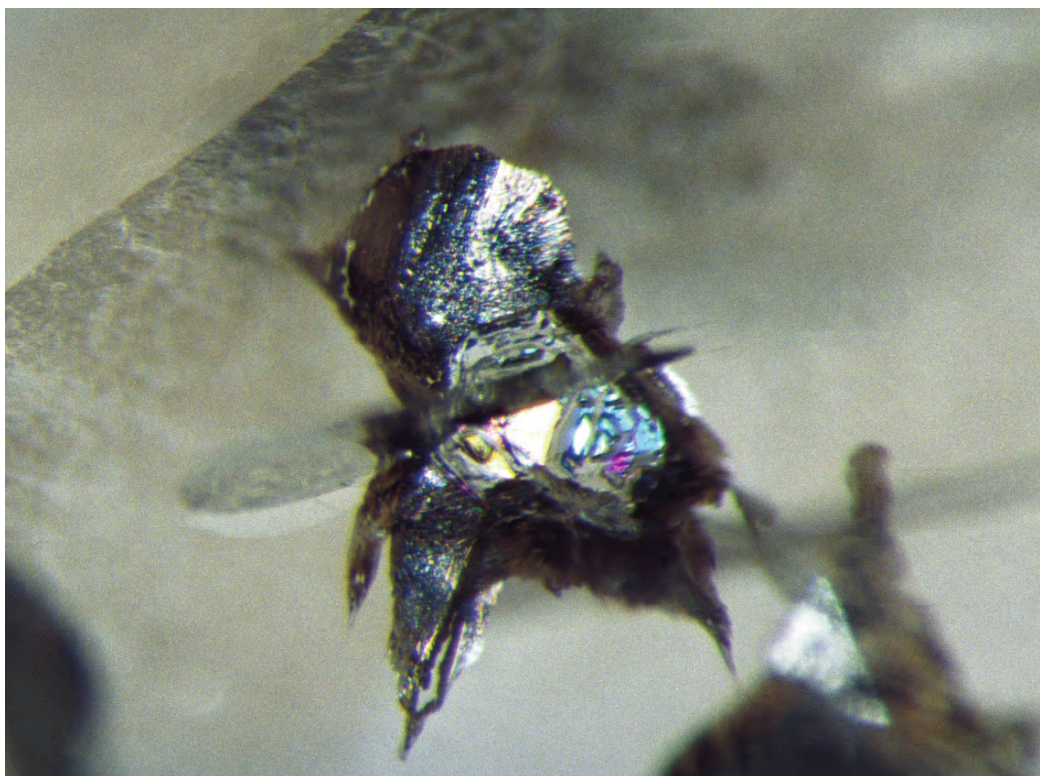
5-29: Inclusion of ferropericlase in a diamond. A fine graphite film on the inclusion-diamond interface probably causes the iridescence. The inclusion is surrounded by graphite coated fractures. The field of view is ~1 mm.
