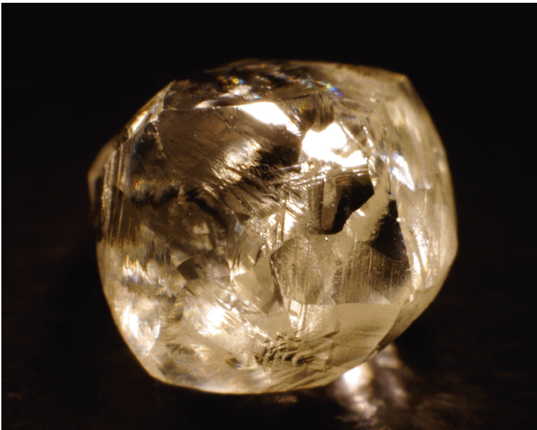
4-30: Colorless dodecahedral diamond with two distinct sets of deformation lines (1.00 ct).
