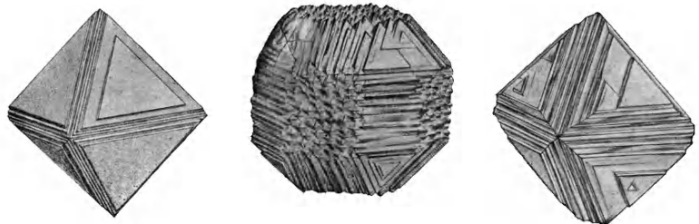
4-03: Octahedral diamonds with triangular growth plates in different configurations. Drawings from Fersmann and Goldschmidt (1911).
