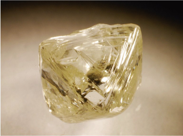
4-06: Rounded triangular growth plates and shield-shaped laminae on an octahedral diamond (1.01 ct).
