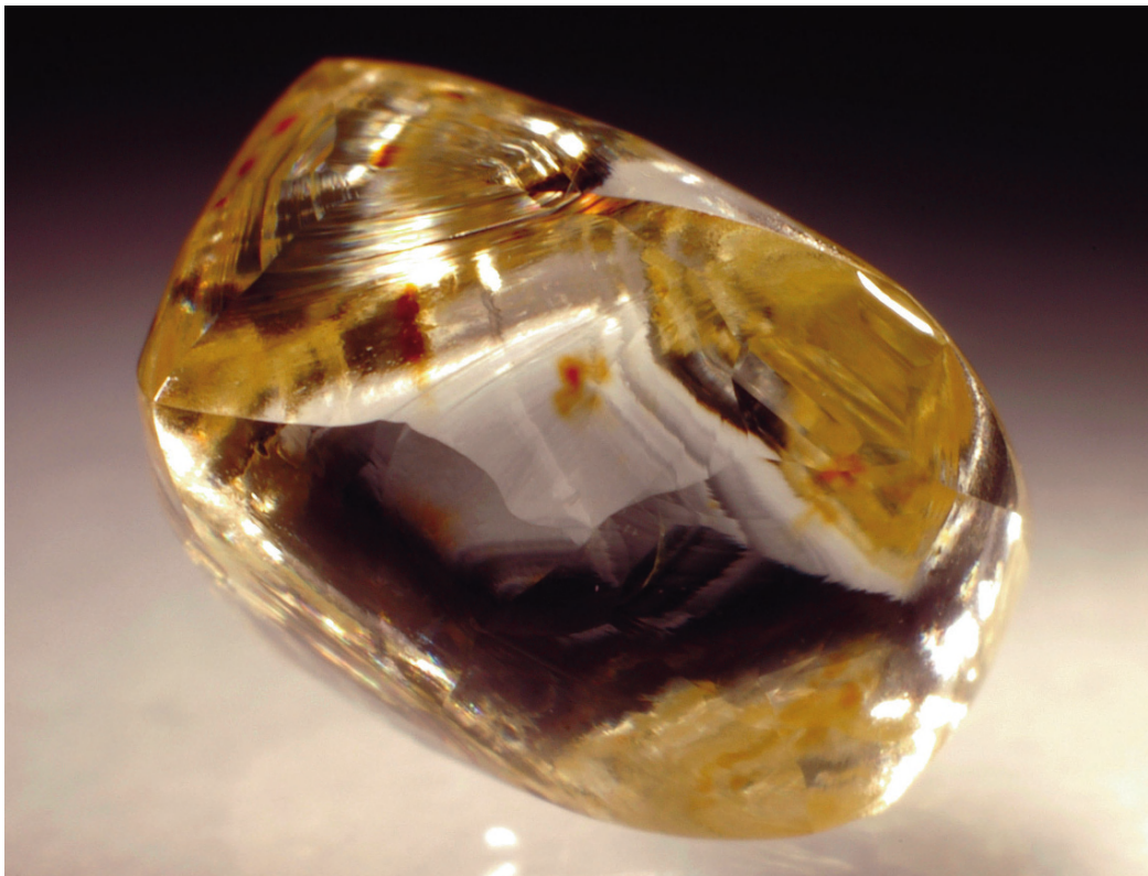
3-01: Transparent yellow diamond with dodecahedral habit (1.02 ct). The pale yellow color, or cape yellow, is typical for Type Ia diamonds. The diamond also exhibits brown irradiation spots.
