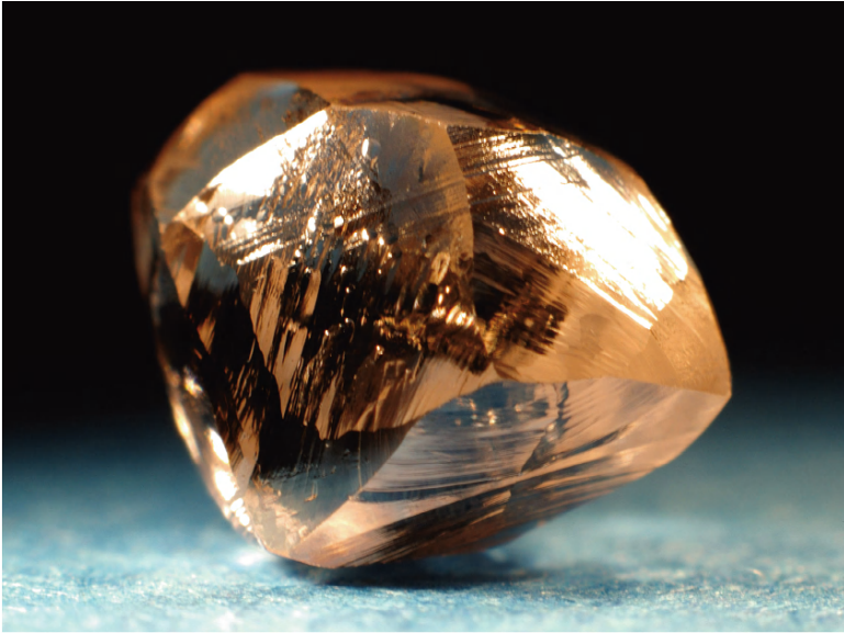
4-29: Left , Brown dodecahedral diamond with two sets of deformation lines oriented in different directions (1.13 ct). The diamond also exhibits elongated hillocks that follow a third direction. Above , Simplified representation of the main crystal faces and the location of the deformation lines (red) and the hillocks (blue).
