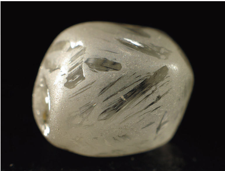
4-44: Abraded dodecahedral diamond (1.10 ct). The deepest parts of the surfaces are not abraded indicating that the diamond was scratched on a hard surface, such as the sidewalls of a pothole within a riverbed.
