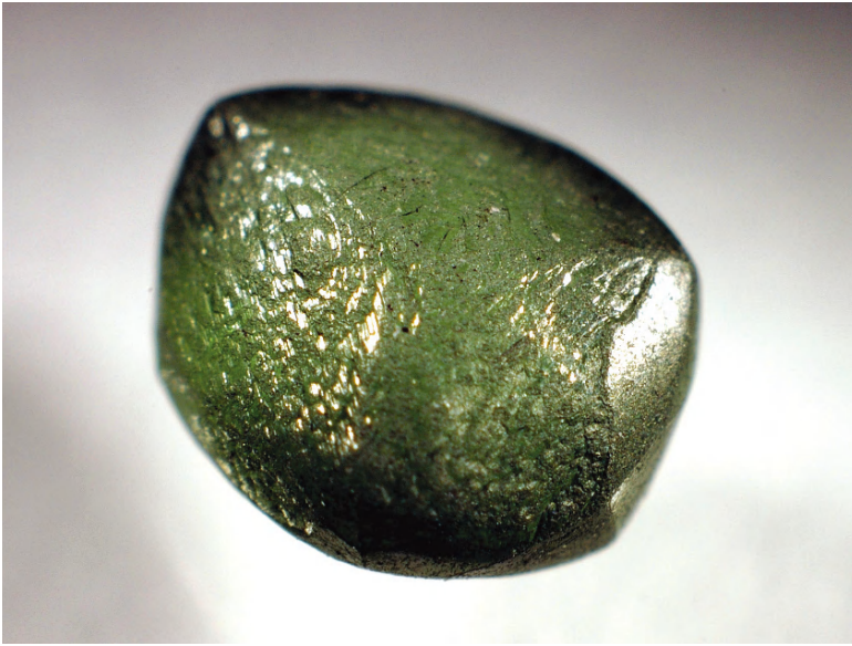
4-35: Coarse frosting on the surface of a rounded dodecahedral diamond with a green surface color (0.32 ct).
