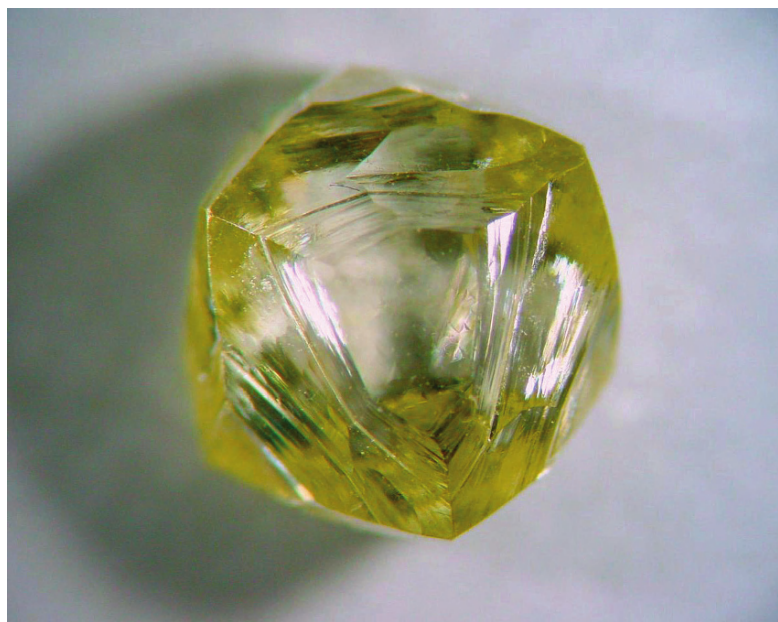
3-13: Slightly elongated dodecahedral diamond with a straw yellow color (cape yellow), which is characteristic for Type Ia diamonds. (1.00 ct).
