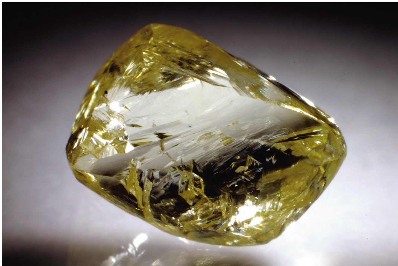
3-13: Slightly elongated dodecahedral diamond with a straw yellow color (cape yellow), which is characteristic for Type Ia diamonds. (1.00 ct).
