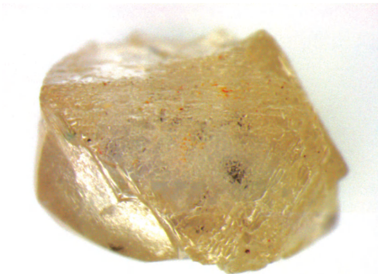
2-23: Left, Pseudohemimorphic diamond from the Springfield Basin, South Australia (0.02 ct). Above, Simplified representation of the main crystal faces showing the rounded dodecahedral (bottom left) and octahedral (right) parts.
