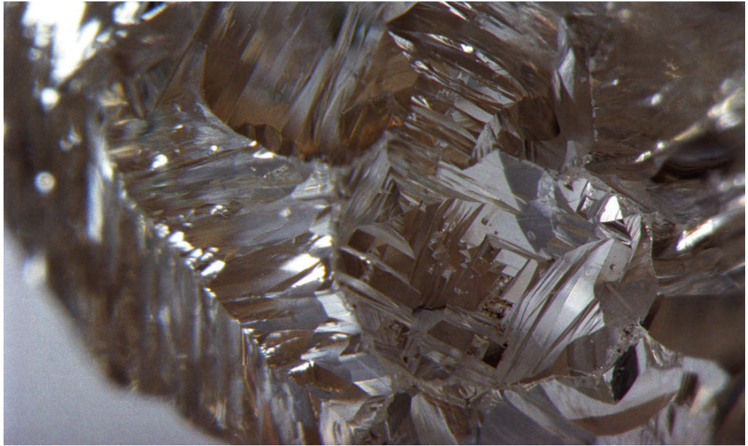
4-14: Deep tetragonal etch pits (tetragons) on the surface of a diamond with a cubic habit. The field of view is ~2 mm.
