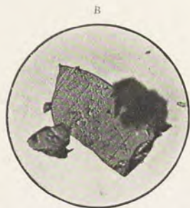
FIG. 21. ARTIFICIAL DIAMOND MADE BY THE AUTHOR FROM MOLTEN IRON.
