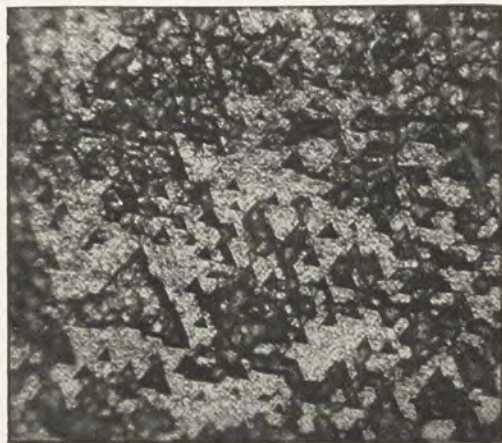
FIG. 16. TRIANGULAR MARKINGS ARTIFICIALLY PRODUCED ON A DIAMOND CRYSTAL.
