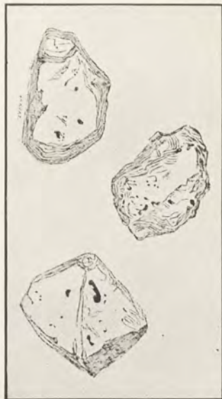
FIG. 22. MOISSAN'S ARTIFICIAL DIAMONDS.
