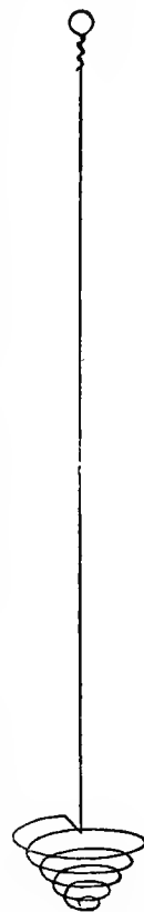
FIG. 2. Basket of platinum wire for holding stone in determination of specific gravity.
