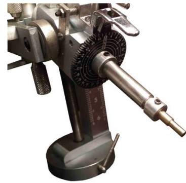
Base Assembly Lock Pull Handle Down to secure Post to Base
