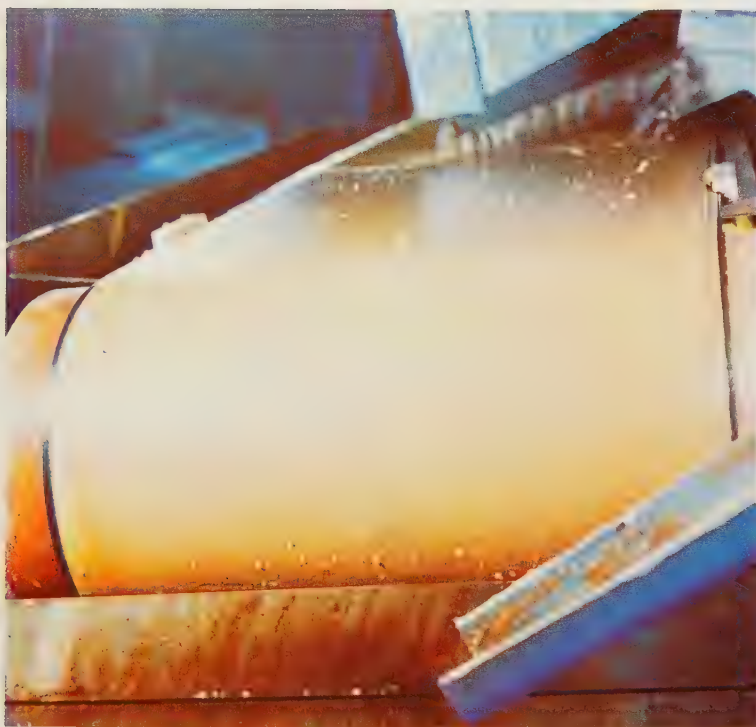
Rough diamonds passing over "greaser" (moving table coated with grease). De Beers.
