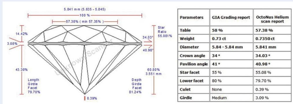
Figure 2.2 The parameters of MSS 13 from its actual Helium Polish scan. This diamond has been used as an actual standard diamond for comparisons of visual and videos for samples of new cut designs.
