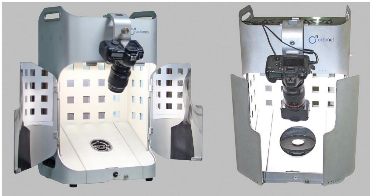
Figure 4.1 On the left is ViBox with the doors open, the Canon DSLR camera and the figure of eight gimbal for holding diamonds. On the right side the doors are partly closed. The stereo splitter has been added to the camera lens and a 360 degree rotating stage is in place.
