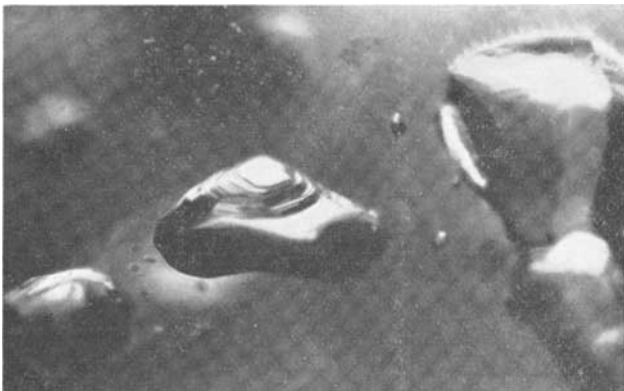
FIG. 11. Ruby from Burma with negative crystals. 190 ×
