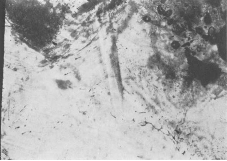
FIG. 2. Gaseous inclusions in the hydrothermal overlayer, which are distinctly separated from the seed by dark pairs of growth lines, which meet at angles. This is distinct and characterizes the natural core, while in the lower part along the demarcation line between the natural crystal and hydrothermal overlayer there are numerous gaseous inclusions. Photo in transmitted light.
