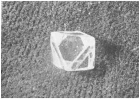
FIG. 8. Photograph of a "glassie" diamond crystal. Taken with an ordinary camera fitted with a 3-dioptre positive lens.
