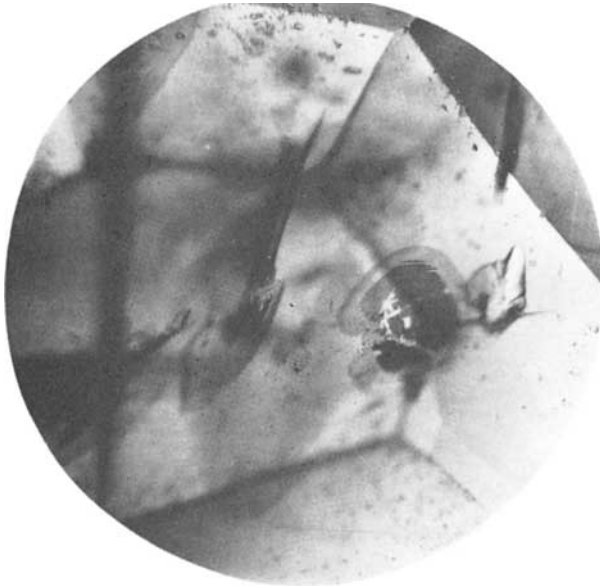
Typical cracks and unpolished facet showing crystal surface, typical of a synthetic emerald-coated beryl
