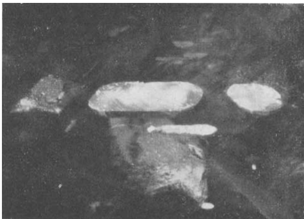
FIG. 5. Corundum in corundum specimen 81721-6, in reflected light (30 ×).
