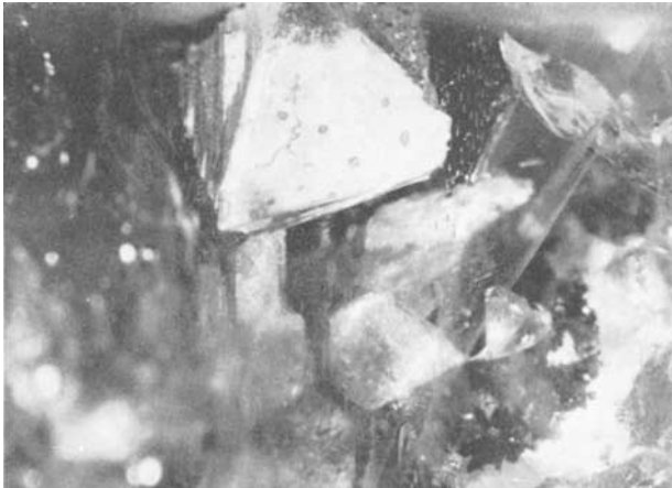
FIG. 4. Spinel octahedron in corundum specimen 81721-4 in reflected light (20 ×).
