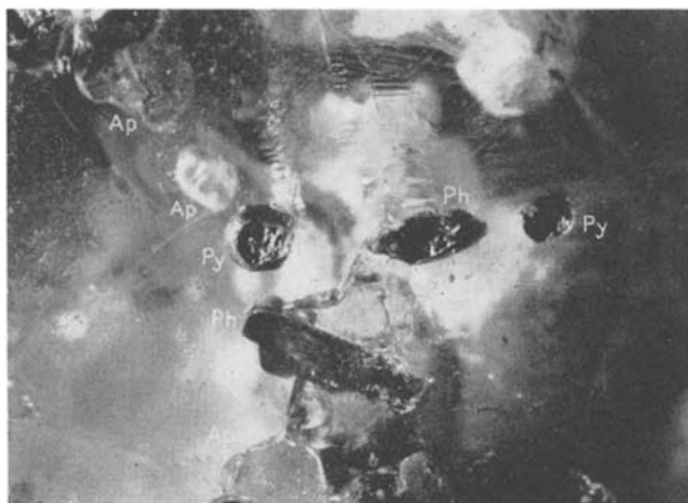
FIG. 2. Pyrrhotite with phlogopite and apatite in corundum. Specimen 81721-2, in both reflected and transmitted light (20 ×).
