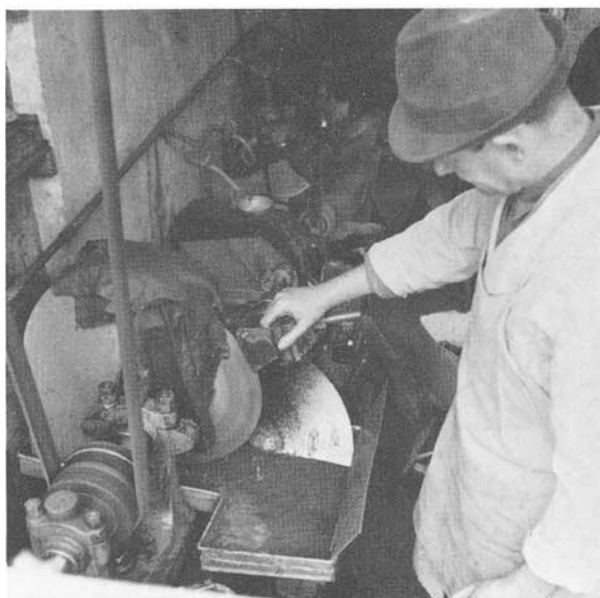
Herr Heinz sawing agate on a copper saw impregnated with diamond dust.
