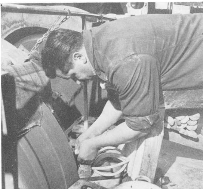
The cutter lies over the saddle holding the agate against the sandstone wheel.
