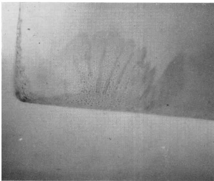
Fan-shaped feathers in low relief seen in a recent synthetic emerald. (Make unknown).
