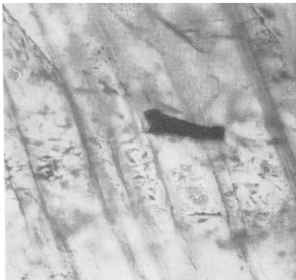
Inclusions in an early hydrothermal synthetic ruby.
