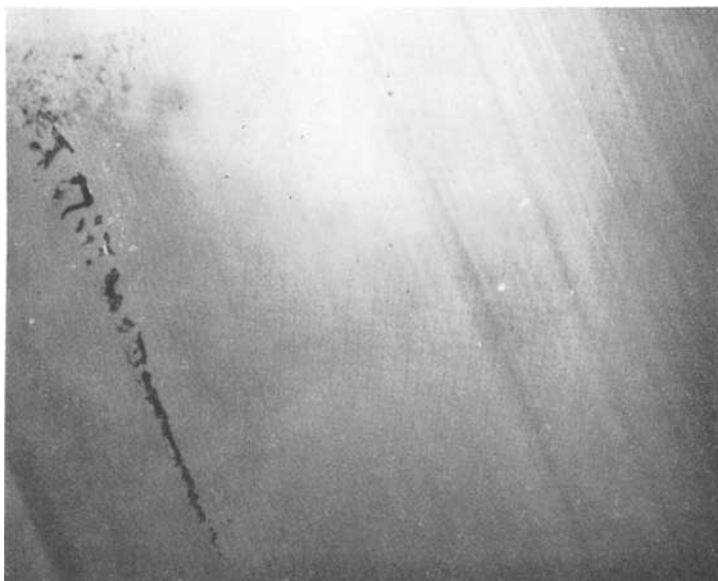
Unusual chain of inclusions and fine straight lines (canals?) seen in a recent synthetic emerald. (Make unknown).
