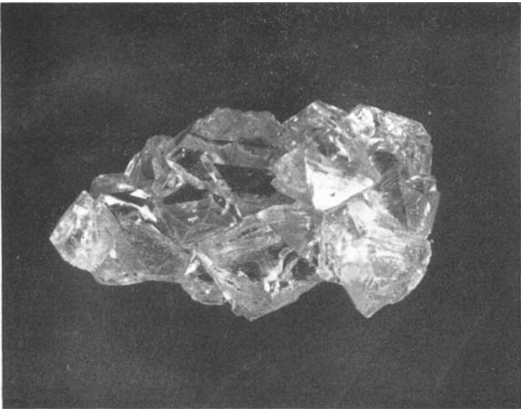
A group of crystals of synthetic spinel grown by the flux-melt method.
