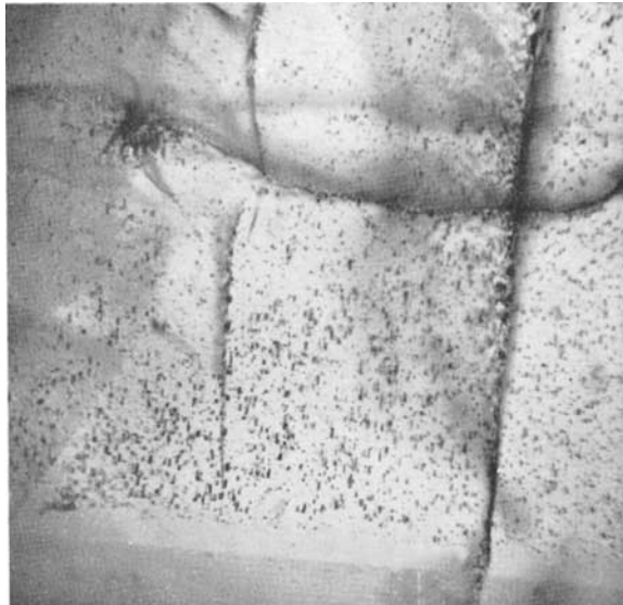
Feathers and rectangular-shaped inclusions seen in a synthetic emerald. (Make unknown).
