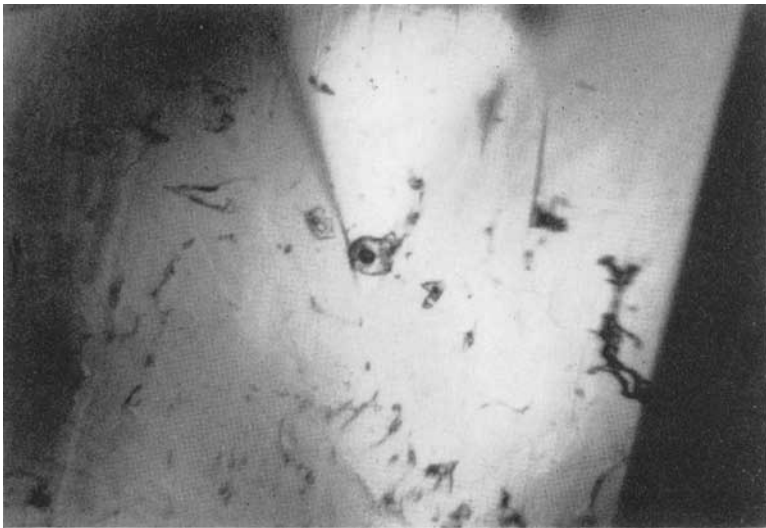
FIG. 4. Colombian emerald 40 \times . Three-phase crystalline lacunae of different appearances and origins. The direction of crystallization is from bottom to top.
