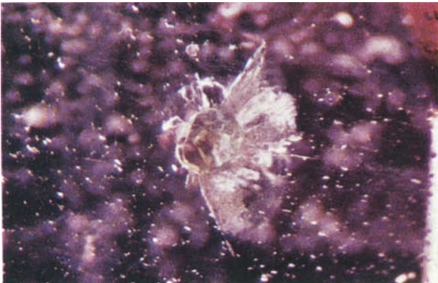
FIG. 7. Transparent, slightly greenish crystal of diopside, surrounded by multiple tension cracks. 16 \times .
