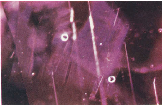
FIG. 6. Clear, transparent, rounded grains of plagioclase, which might easily be mistaken for gas bubbles when observed in an otherwise pure Siam ruby. 16 \times .
