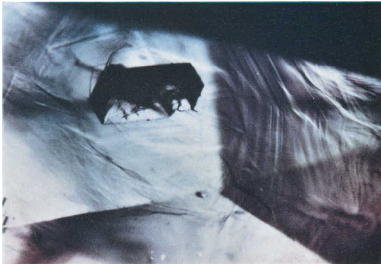
FIG. 3. Colombian emerald 40 \times . Calcite crystal causing intense coloured growth disturbance.
