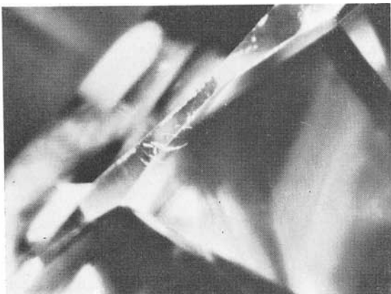
FIG. 7. 1.69 carat diamond. Flawed girdle: separate fissures seen. (25 ×).
