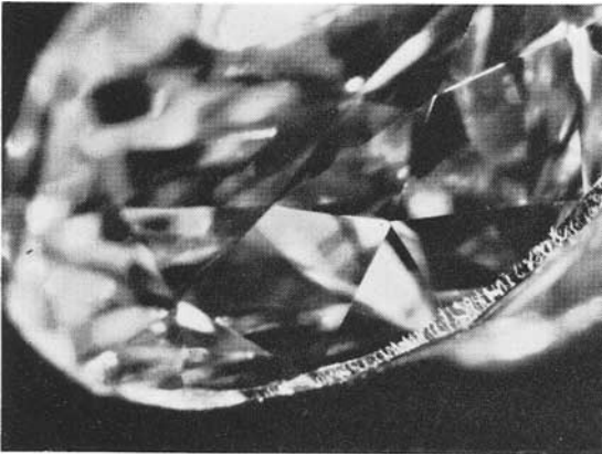
FIG. 3. 1.05 carat diamond with a flawed girdle, seen from a side (10 \times ).
