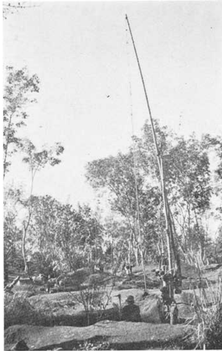
FIG. 2. A bamboo crane used for lifting soil from the mine shafts.
