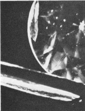
FIG. 5. Three-phase inclusion; octahedral and tube inclusions. 30 \times .
