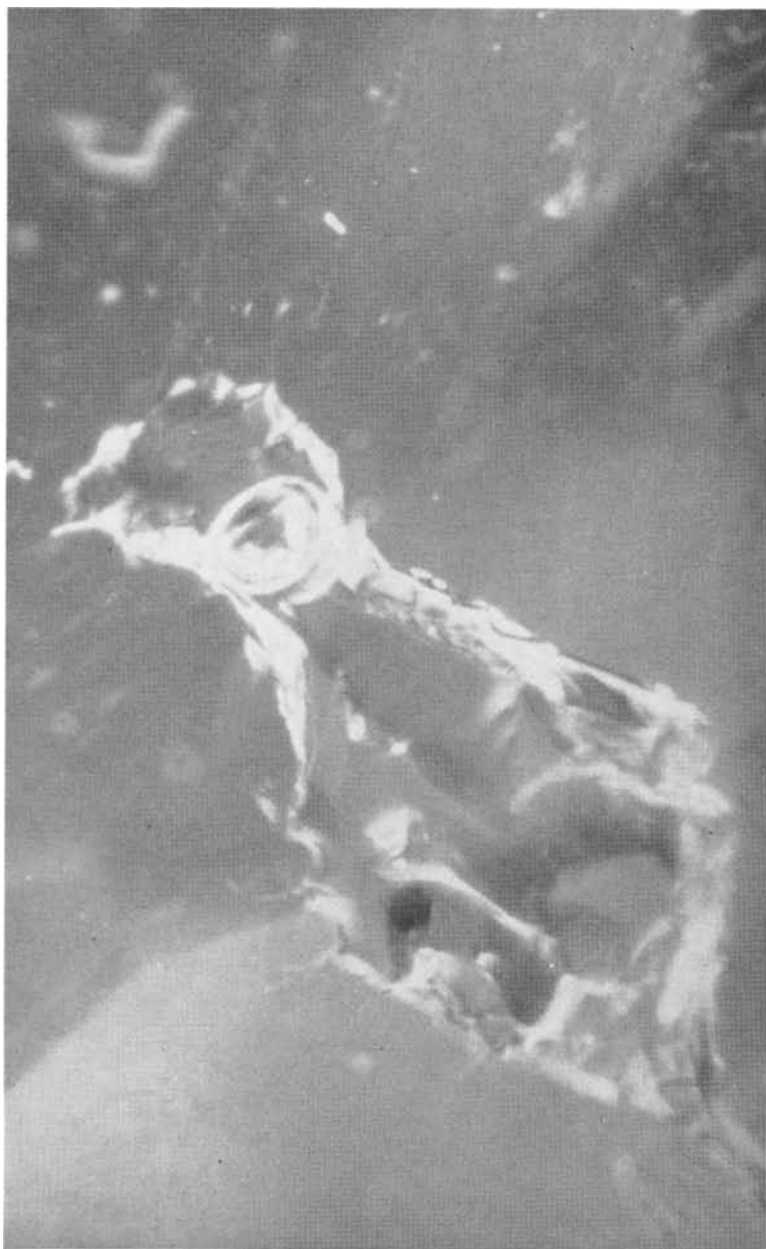
FIG. 2. Two-phase irregular inclusion in beryllonite from Stoneham, Maine. (N.M.N.H. gem #423). (40 \times ).
