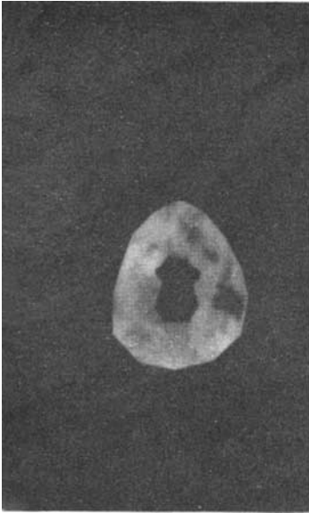
FIG. 2. Contact immersion photograph taken by short-wave ultraviolet light, showing the total light transmission through the two parallel facets (above and below), but only partial transmission elsewhere due to internal reflections by the many other facets. Same size.
