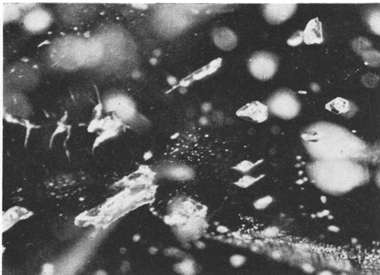
FIG. 5. Adjacent occurrence of primary and pseudo-secondary mono- and bi-phase inclusions in blue topaz. 45 ×
