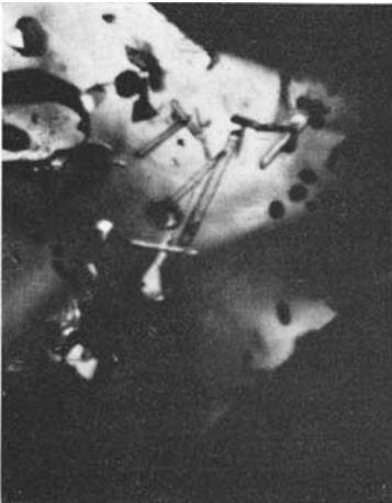
FIG. 9. Angular platelets and two-phase inclusions in a Chatham synthetic ruby.
