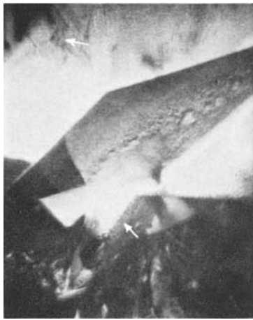
FIG. 2. Gas bubbles at the junction of two Chatham synthetic sapphire crystals and fine-line angular zoning.
