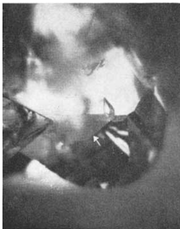
FIG. 1 A frosted area seen on the base of a group of Chatham blue synthetic sapphire crystals.
