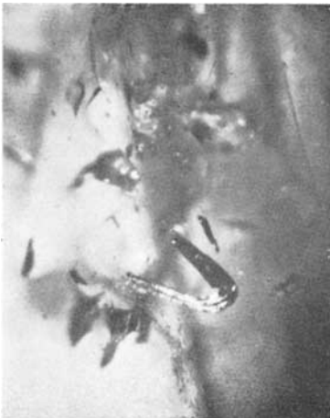
FIG. 5. A U-shaped inclusion, angular platelets, and a few needle-like inclusions in a Chatham synthetic sapphire.
