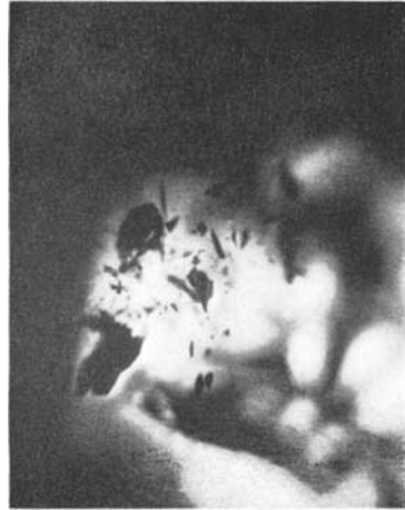
FIG. 6. Angular platelets in the Chatham synthetic sapphire.
