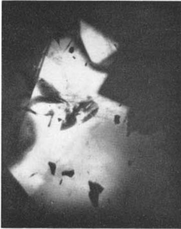
FIG. 7. Angular platelets in the Chatham synthetic sapphire.
