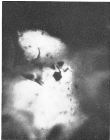
FIG. 10. Angular platelets in a Chatham synthetic ruby.
