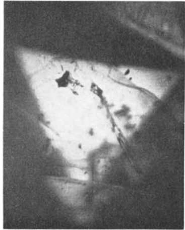
FIG. 4. Two-phase inclusions, veil-like feathers and a few small angular platelets in the Chatham synthetic sapphire.
