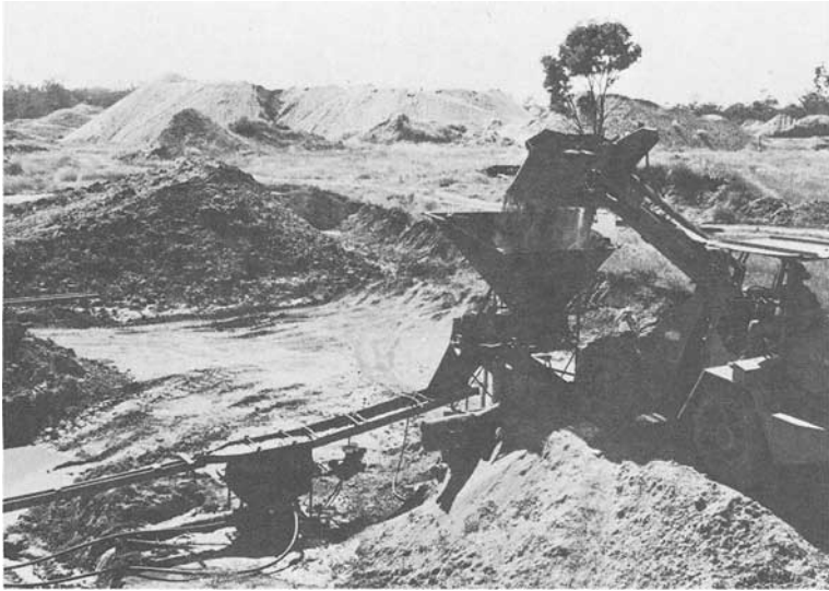
Fig. 3. Excavation and processing the gravel from the Scrub Lead field south-east of Rubyvale. The sapphire-bearing gravel is excavated from the pits and dumped into a sieve, sluice and pulsating jig sequence to gravity-separate the heavy gemstones.
