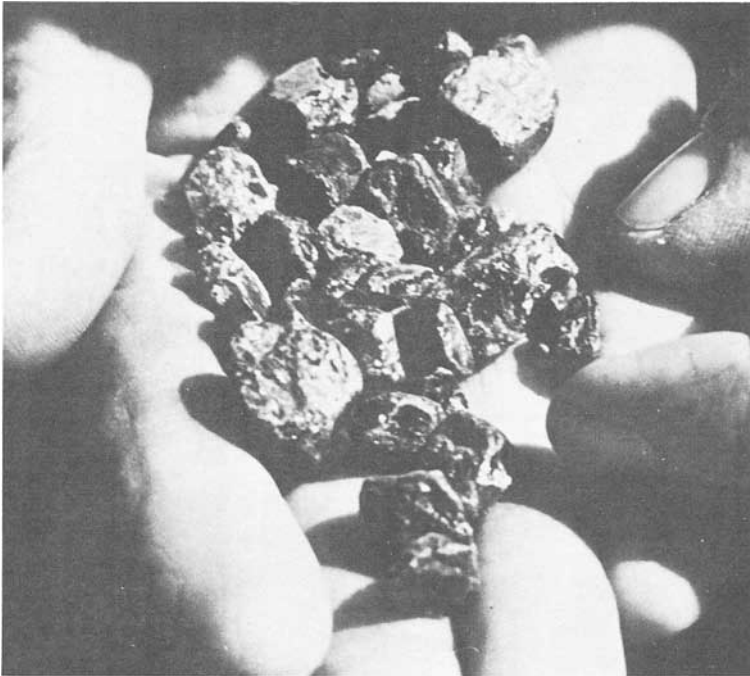
Fig. 6. An ounce of mine-run blue sapphires from the Scrub Lead. Note the angular shapes and poorly preserved crystal and cleavage faces.
