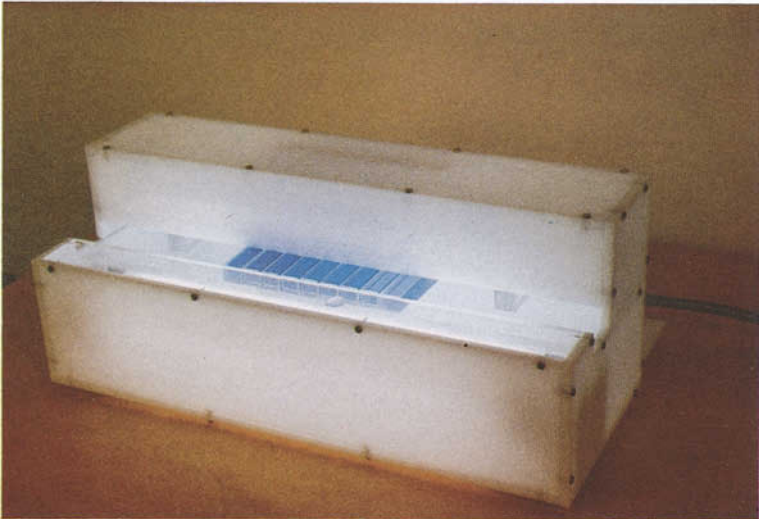
FIG. 13. Light box with lid closed. Comparison colour grading is effected on the transparent section in front of the cuvettes.
