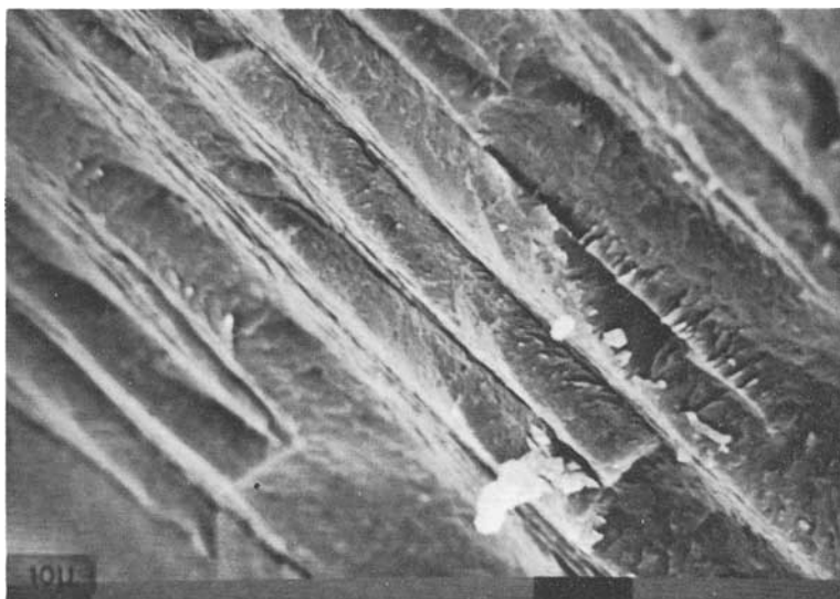
FIG. 2. S.E.M. Photograph of Whitby jet showing woody structure.
