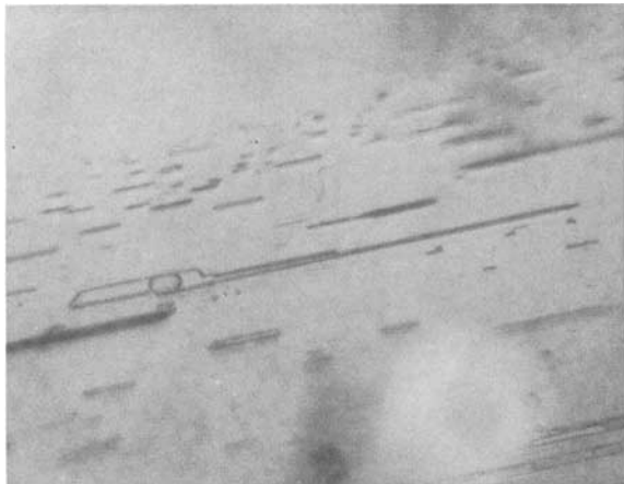
FIG. 1. Elongated two-phase inclusions in diaspore.
