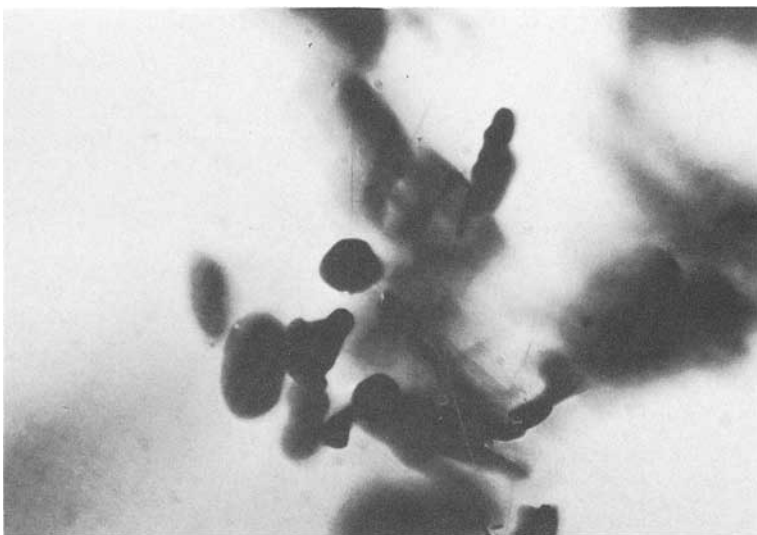
FIG. 13. Black, opaque, thin tabular crystals with a somewhat hexagonal outline. 200 \times .
