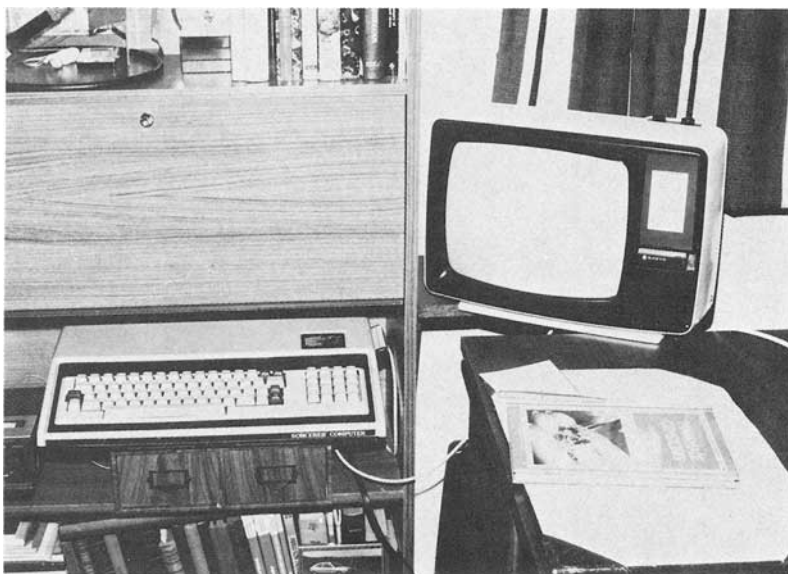
FIG. 1. The author's installation. On the left of the computer is a small domestic tape recorder which is used to feed in the GEM DATA programs.
