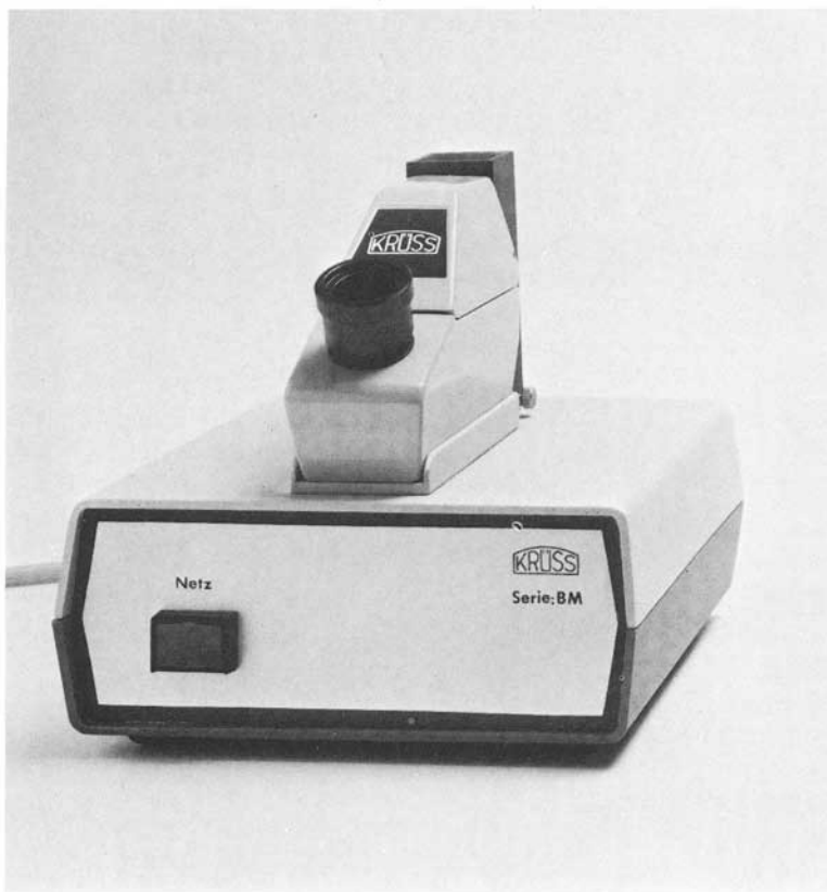
FIG. 1. The Krüss Riplus ER602 refractometer uses a heated strontium titanate prism and a special contact paste. Its measuring range is 1.79 - 2.21
