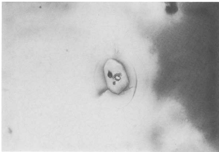
FIG. 4. Thin tabular crystal inclusion, surrounded by a single halo, in garnet from Finland. (180 \times )
