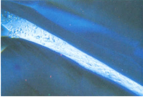
FIG. 33. Scabs on the surface of the reflecting half of a 'double girdle', indicating that this sapphire was heat treated. 25 ×
