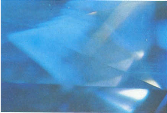
FIG. 40. Phantom-like cloud enhanced by thermal heat treatment. 32 ×
