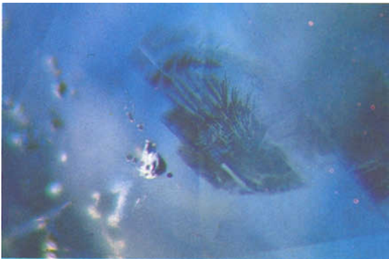
FIG. 44. Fracture, open at the surface of a diffusion treated sapphire, dyed deep-blue by penetration of the dye. 16 x
