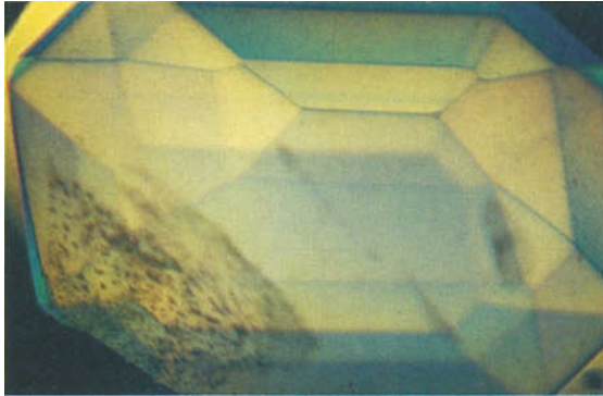
FIG. 48. Diffusion treated sapphire immersed in methylene iodide showing strong blue relief of facet edges and girdle. 16 ×
