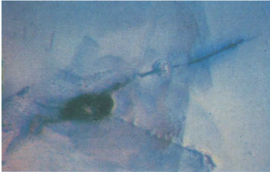
FIG. 46. Enhanced coloration of an inclusion cut flush with the surface of a sapphire diffusion treated for colour alteration. 50× (Photo by C. A. Schiffmann, Gem Laboratory Gübelin)
