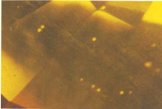
FIG. 37. Typically fringed perimeter of an inclusion modified by heat treatment. 64 ×
