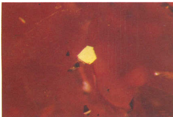
FIG. 27. Hexagonal platinum platelet reflecting the impinging light with a metallic silvery lustre. 25 ×
