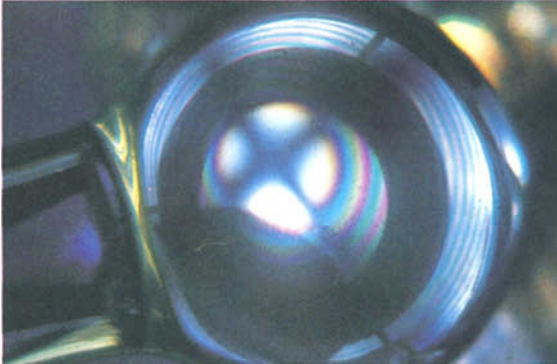
FIG. 2. Sapphire crystal in same position as in Fig. 1. The conoscopical image of the optical monoaxis passing vertically through the basal plane is made visible by a glass ball between crossed polars. 10x
