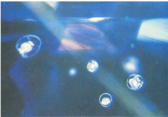
FIG. 35. Tell-tale inclusion scene consisting of several 'cooked' mineral inclusions surrounded by circular lace-fringed fractures. 32 ×
