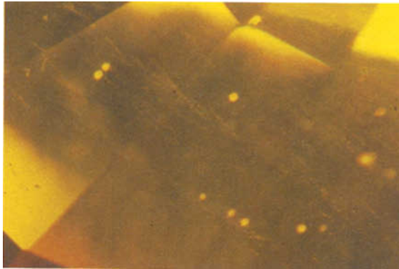
FIG. 41. Unambiguous appearance of the interior of a heat treated yellow sapphire: rounded 'cooked' mineral inclusions amidst striped 'fog' causing turbidity. 25 ×
