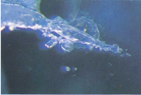
FIG. 7. Coarse formation of flux inclusion. 40 ×
