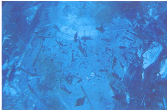
FIG. 21. Flux-grown sapphire by Chatham teeming with platinum inclusions of various shapes (hexagonal, triangular and rectangular platelets, rods, spikes, splinters, etc.) 8 ×
