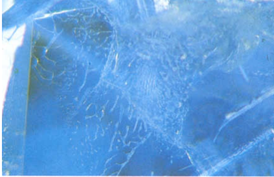
FIG. 13. A loosely designed 'fingerprint' inclusion superposed by a 'feather' of dense lace-like flux-remnants. 20 ×
