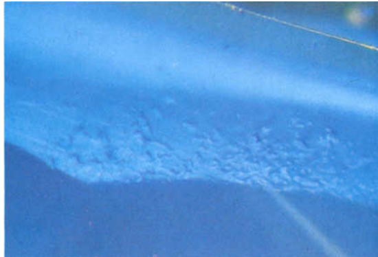
FIG. 34. Pockmarked upper half of a 'double' girdle on a heat treated, sapphire. 40 ×
