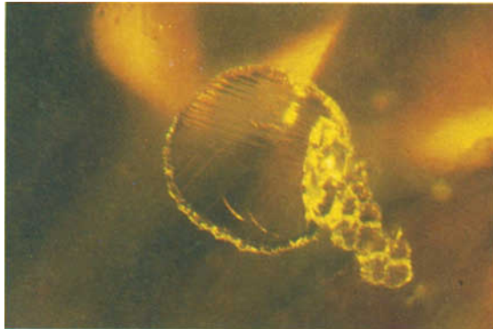
FIG. 38. Unusual cluster of molten mineral inclusions in contact with a circular tension fracture in front of zonal turbidity in a heat treated yellow sapphire. 40 ×
