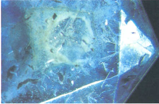
FIG. 1. Synthetic flux-grown sapphire by Chatham. Tabular crystal with large basal plane surrounded by triangular rhombohedra. Note greenish core. 8x
