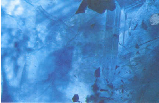
FIG. 4. Characteristic inclusion scene in synthetic sapphire by Chatham, comprising angular zones, tiny flux grains and black platelets of platinum (one of them in the top right-hand corner with silvery reflection). 15 ×
