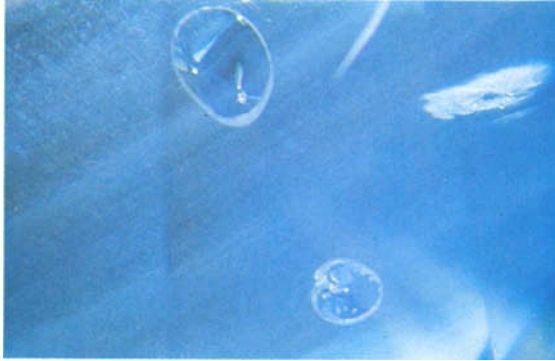
FIG. 36. Characteristic appearance of the interior of heat-treated sapphires: turbid zones encompassing white, dusty particles and typically atoll-like inclusions (the one near the upper right-hand corner shows high reflection). 25 ×
