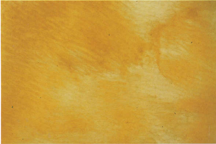
FIG. 2. Gem microscopic examination using high intensity fibre-glass optic light showing 'chicken wire' appearance. (transmitted light. 20 \times )
