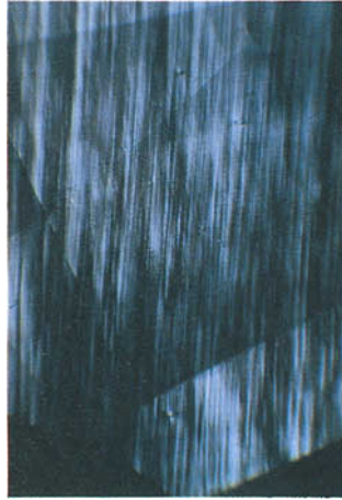
FIG. 10. Part of diamond viewed between crossed polars and showing strain birefringence resembling albite (feldspar) twinning.
