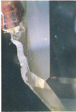
FIG. 9. Corner of diamond showing re-drilled support hole and traces of former hole.
