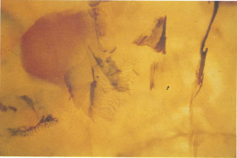
FIG. 4. Often visible red colour-patches and typical dendritic patterns seen in the Gilson imitation. (transmitted light. 20×)
