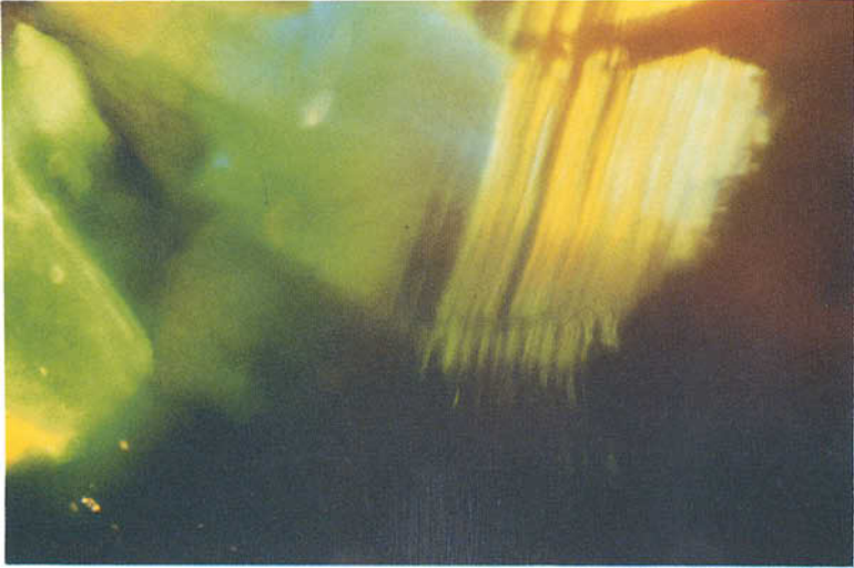
FIG. 6. The structural pattern seen in most of the colour segments of natural honey opal. (transmitted light, 40 ×)
