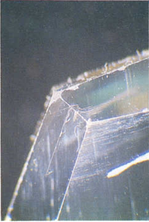
FIG. 8. Part of 56.71 ct diamond showing cleavage traces in two directions and scratch 2.5 mm long.
