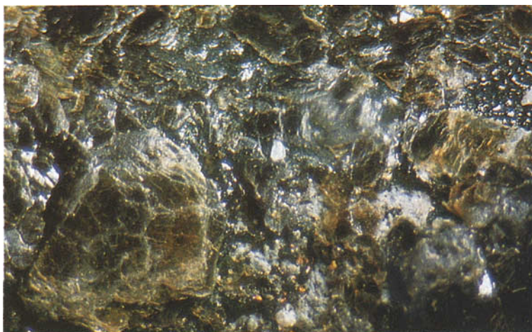
FIG. 3 The mica adhering to the surface of the imitation crystal in Fig. 2.
