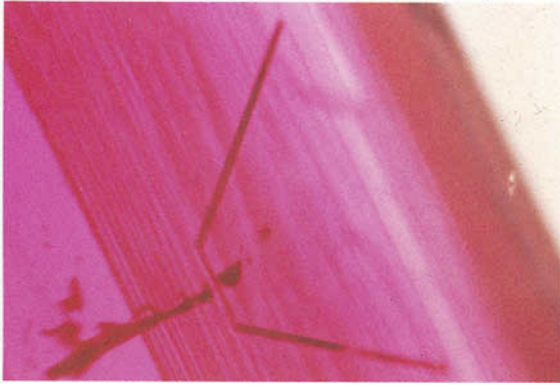
FIG.10. Orientation of secondary dense flux in a random direction to that of the preliminary concentrated flux. The drippy appearance of the flux can also be noted. (dark-field illumination) 40 × .
