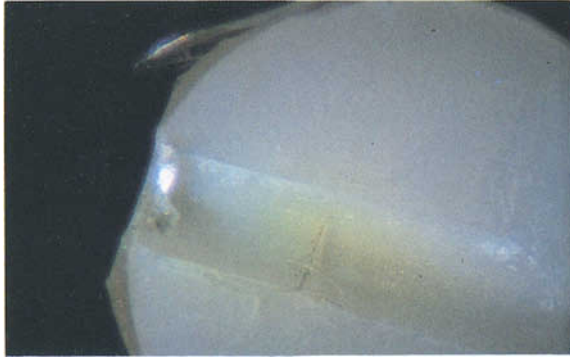
FIG. 30 A sliced 'Angelo' imitation pearl showing the shell bead centre and the thickness of the outer layer.
