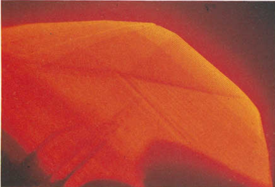
FIG. 5. Straight growth phenomenon seen under the immersion microscope using methylene iodide ( n_D = 1.74 ) and a narrow beam of light. 20\times .
