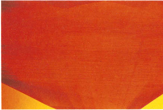
FIG. 7. Graining observed from girdle to girdle in the new synthetic ruby from U.S.A. (immersion microscope) 22 \times .
