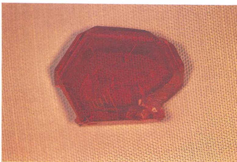
FIG. 2. A tabular crystal of Ramaura synthetic ruby weighing 7.46 carats.
