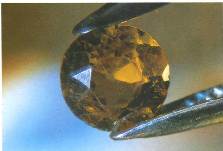
FIG. 5 The same natural sapphire as seen in Fig. 4 after a ten-minute exposure to x-rays.
