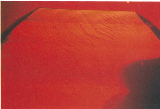
FIG. 6. Diagnostic 'hallmark' of Ramaura flux ruby 'Scotch in water' or 'heat wave' effect. (immersion microscope) 25\times .
