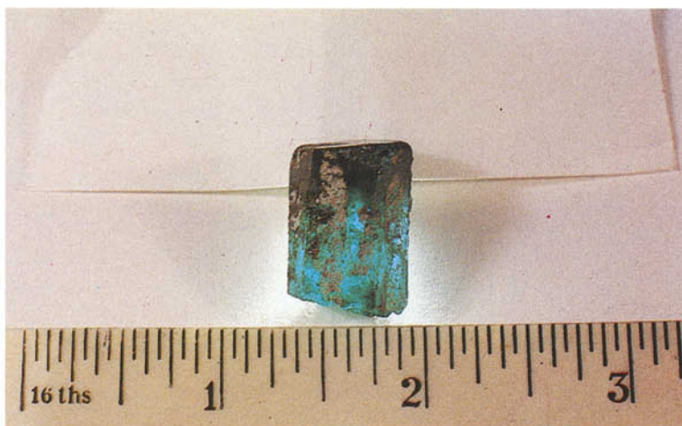
FIG. 2 An imitation emerald crystal made of glass and with mica adhering to its surface (see Fig. 3).
