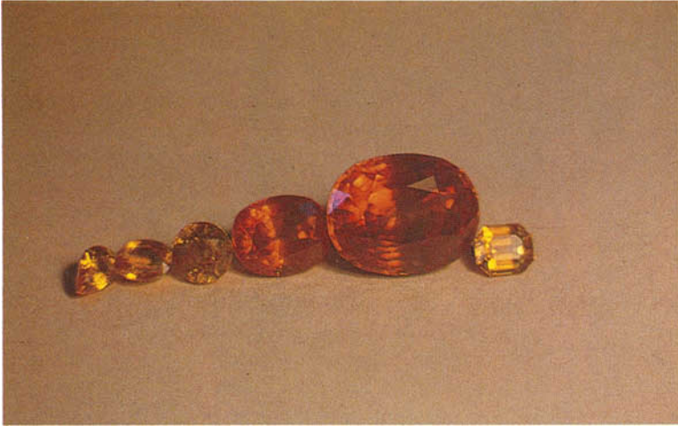
FIG. 6 Four small heat-treated yellow sapphires and two large orange sapphires which owe their colour at least partly, if not wholly, to heat treatment.
