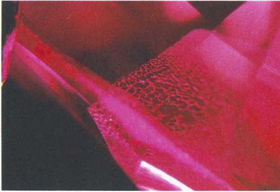
FIG. 16. The lace-like flux feather with diagnostic clear-cut appearance frequently seen in Ramaura flux ruby. (dark-field illumination) 30 \times .
