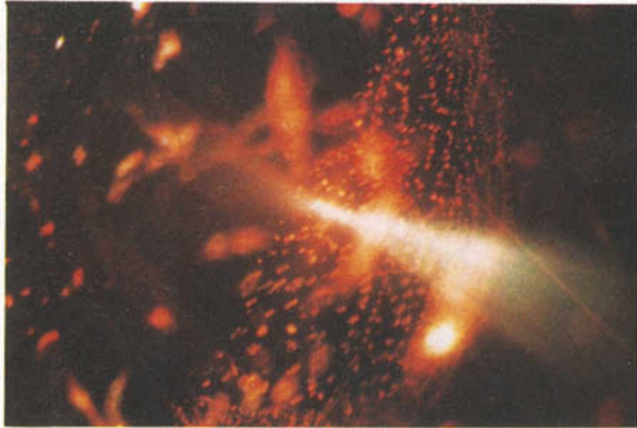
FIG. 2. Typical feather of crystallites, another common feature in reddish-brown sapphires of Tanzanian origin. 40x . (dark field illumination).
