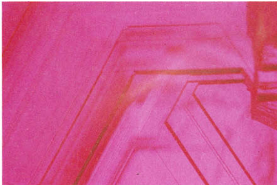
FIG. 9. Orientation of tube-like dense flux parallel to the pseudo-hexagonal zonal lines. Note the uneven colour concentrations. (dark-field illumination) 60 \times .
