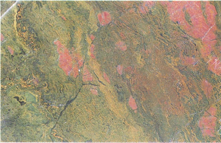
FIG. 4. Close-up of banding and of irregular patches of fine-grained ruby in verdite, Zimbabwe. Red-ruby, green-chromian muscovite, brown-hydrated iron oxides, arsenates and other minerals.
