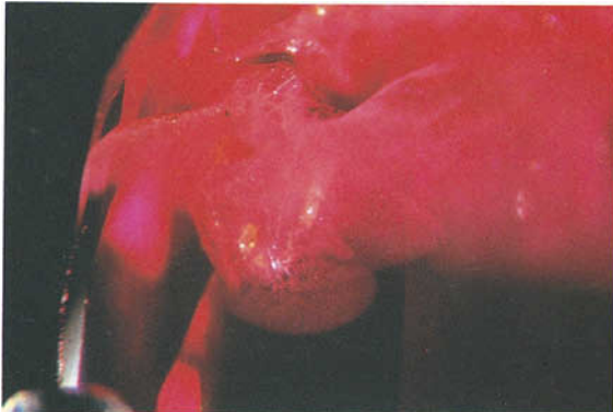
FIG. 12. Orange-yellow flux globules with radiating fine flux leathers in Ramaura product. (dark-field illumination) 35 × .
