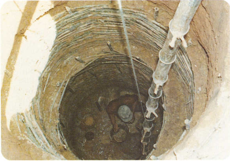
Figure 3. Pit mining of sapphires in Bo Phloi. The walls of the pit are reinforced with bamboo canes and the 'bamboo ladder' used to climb down to the pit.
