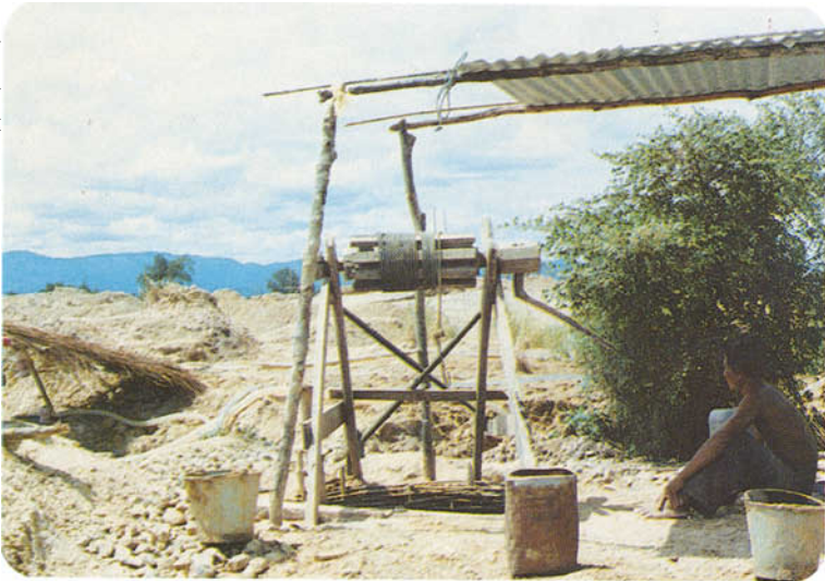
Figure 4. Hoisting the buckets containing the gem gravel by means of crude pulley-type mechanism.
