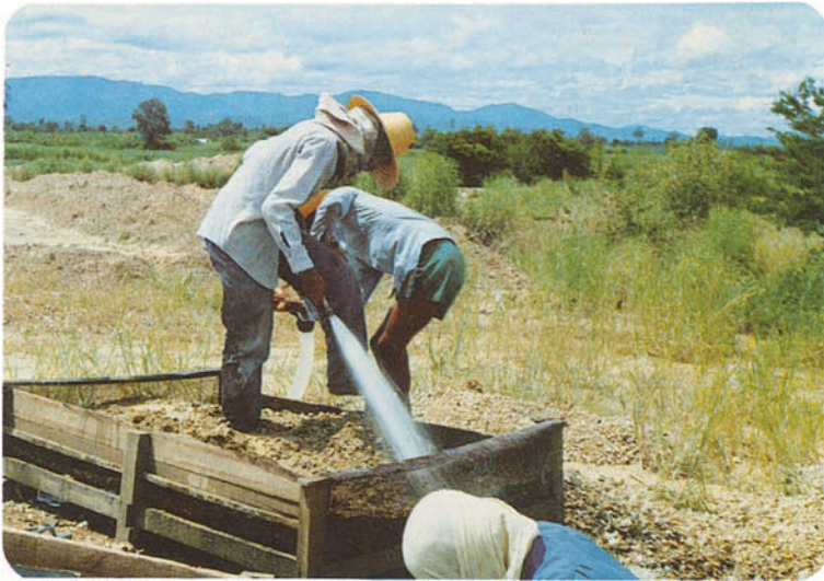
Figure 5. Use of strong jets of water to clean the remaining clay at the final stage of cleaning. Later, the workers sit on these large wooden crates and pick out the sapphire crystals by hand.
