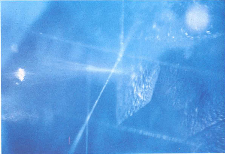
Figure 10. Needle-like structures of dislocation directions are frequently seen in sapphires from this locality. 25 ×. (photo: M. Gunawardene)
