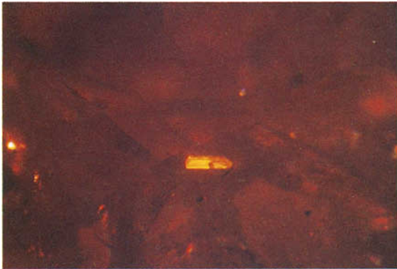
FIG. 16. Short, stubby plate-like prisms seen in an Inamori -grown synthetic orange sapphire. (reflected light, 32 \times ).
