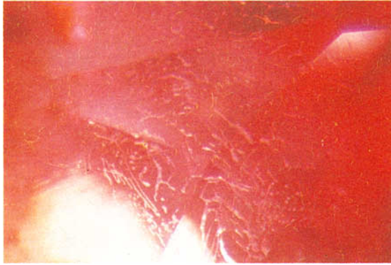
FIG. 6. Scenery of a lace-like flux feather in Chatham -made synthetic orange sapphire. (darkfield, 35 \times ).
