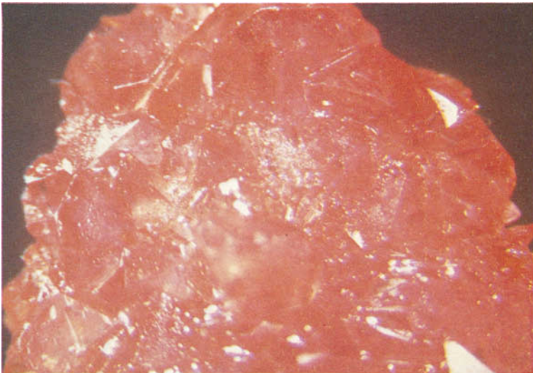
FIG. 1. A crystal cluster of flux-grown synthetic orange sapphire marketed by Chatham Created Gems, Inc. , San Francisco, U.S.A. (10×).
