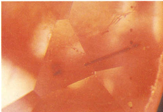
FIG. 17. Needle-like platinum inclusions with dull metallic lustre, embedded in a flux-grown synthetic orange sapphire made by the San Francisco firm. (transmitted light, 30 \times )
