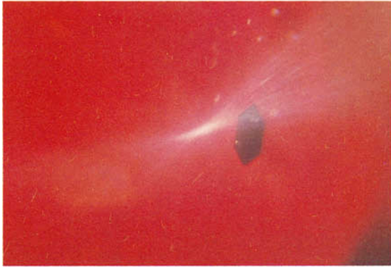
FIG. 15. The platinum plate in Figures 13 and 14 now observed from the side. It appears very thin as usual like the plate-like inclusions. (transmitted light, 50 \times ).
