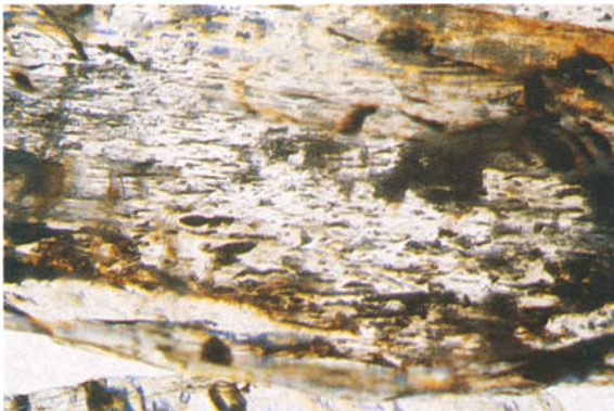
FIG. 8. Colourless enstatite, Sri Lanka. Healing fractures indicated by iron oxide surfaces, brownish micaceous laminae, and minute two-phase inclusions. \times 15 .
