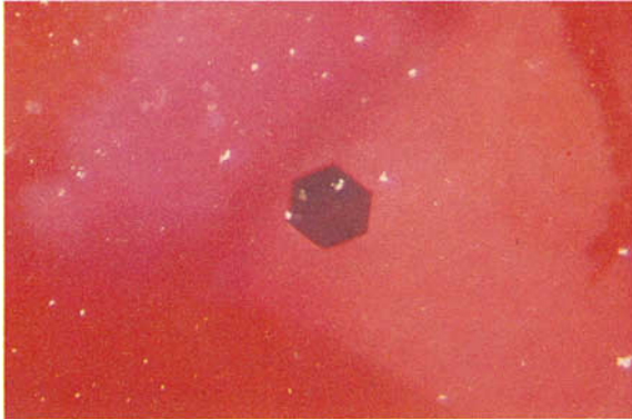
FIG. 13. Pseudo-hexagonal outward appearance of a platinum inclusion enclosed in a Chatham flux-grown orange sapphire. (transmitted light, 46 \times ).
