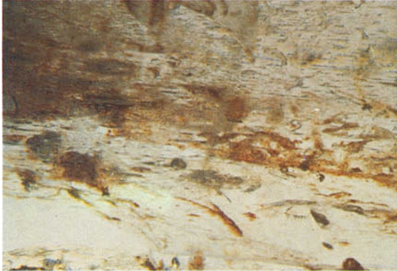
FIG. 10. Colourless enstatite, Sri Lanka. Healing fractures indicated by irregular iron oxide surfaces and elongated minute two-phase cavities. Brassy single crystals of pyrite are present. \times 8
