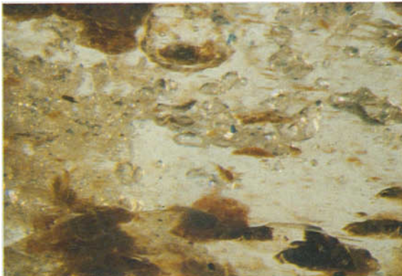
FIG. 5. Colourless enstatite, Sri Lanka. Iron oxides are localized in the brownish-red areas; also present are colourless transparent crystals of quartz. \times 15 .
