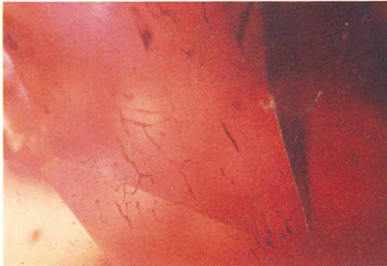
FIG. 10. General view of the new synthetic orange sapphire manufactured by Chatham . Flux inclusions, patchy coloration of yellowish-orange, orange and pinkish-purple areas and platinum inclusions. (darkfield and lightfield, 32 ×).
