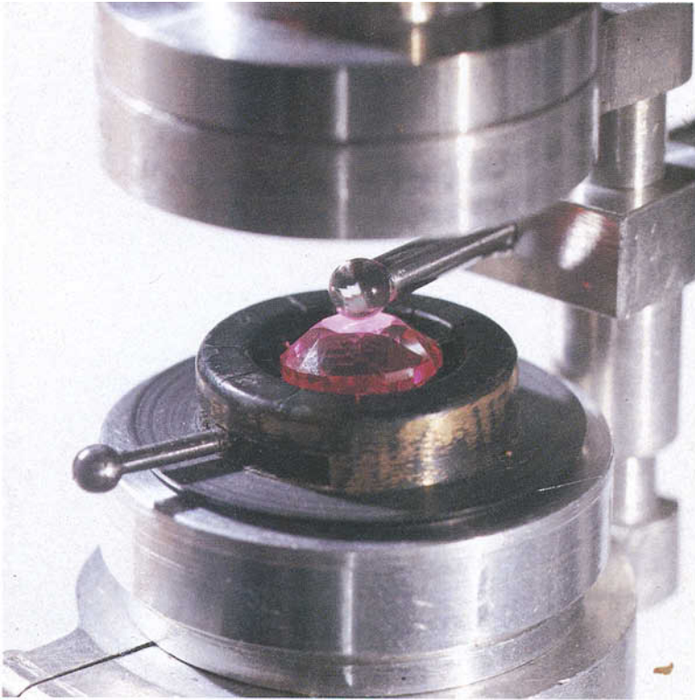
FIG. 6. Enlarged view of the conoscope condenser arm.
