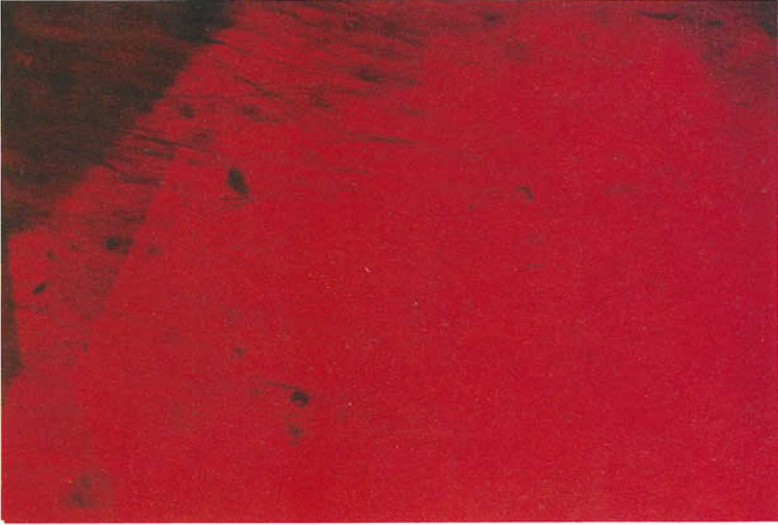
FIG. 4. Comet- or hairpin-like melt residue inclusions in a synthetic Kashan ruby. (28 × )
