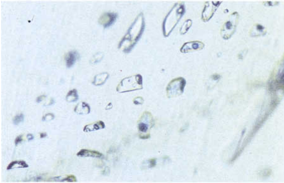
FIG. 2. Parallel alignment of two- and three-phase negative inclusions.
