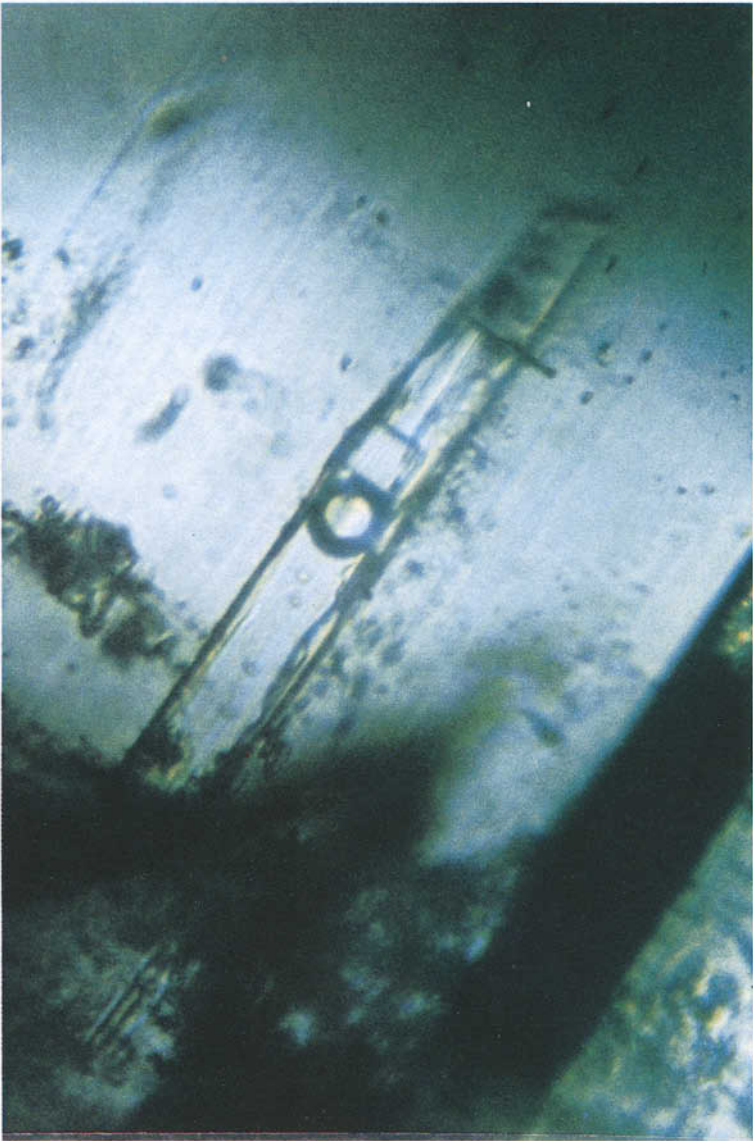
FIG. 1. Needle-like cavity with a liquid, a gas bubble and a crystal, forming a 'three-phase-inclusion' in a South African emerald (400x)
