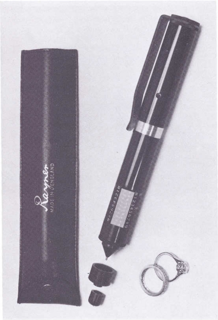
FIG. 1. View of the Rayner DiamondScan showing (centre, right to left) its bar-graph type indicator, stainless steel test tip, removable test platform and dust cap.
