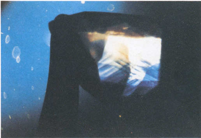
FIG. 4. 'Plato striation' obtained parallel to the c axis while the stone was immersed in methylene iodide between crossed polaroids in their dark position. (15 ×)
