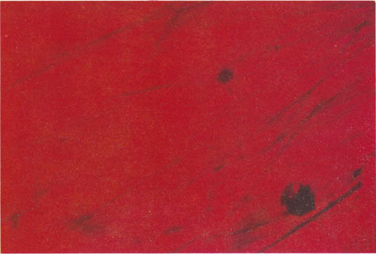
FIG. 5. Comet- or hairpin-like melt residue inclusions in a synthetic Kashan ruby. (50 × )
