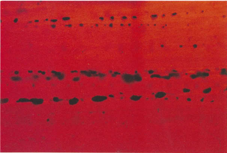
FIG. 3. String of pearl-like inclusions of melt residues in a synthetic Kashan ruby. (50 ×)
