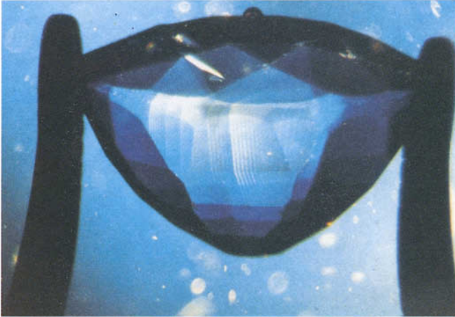
FIG. 3. Polysynthetic twin lamellae in Verneuil synthetic with interference rings along the twin planes as seen while the stone was immersed in methylene iodide between crossed polaroids. (15 ×)
