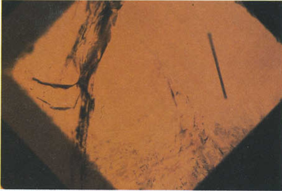
FIG. 4. The same fracture system using partial immersion and transmitted light. Notice the single tiny acicular diopside inclusion. 40 × .
