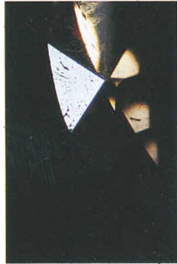
FIG. 10. Surface cavities on the host corundum during the overgrowth procedure in Lechleitner coated synthetic corundums. Reflected illumination . Magnified 22x.
