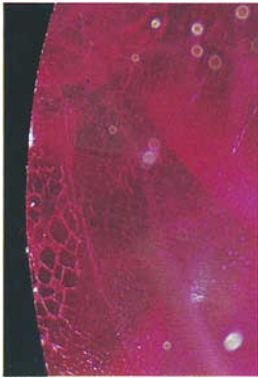
FIG. 12. Very fine 'nets' revealed in Lechleitner coated synthetic ruby. Dark-field illumination . Magnified 32x.
