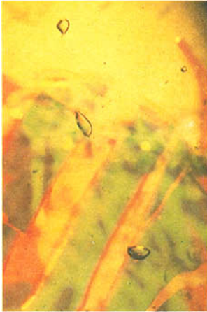
FIG. 7. Three normal bubble shapes showing high relief. Green flakes in background. Fire opal simulant. 10x.
