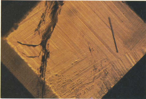
FIG. 5. Shadowing is now used and the garnet's rhombic dodecahedral-trapezohedral structure becomes visible. 40 × .
