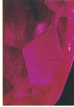
FIG. 19. Feathers (resembling those seen in heated natural rubies) observed in Lechleitner coated synthetic ruby. Dark-field illumination. Magnified 35x.
