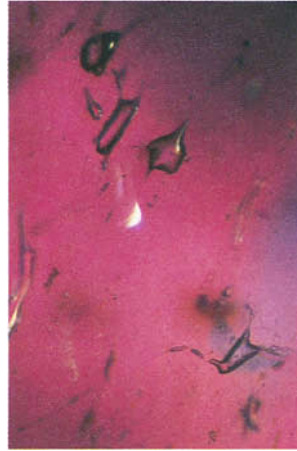
FIG. 13. High relief bubbles with spiky terminations. Black opal simulant. 42x.
