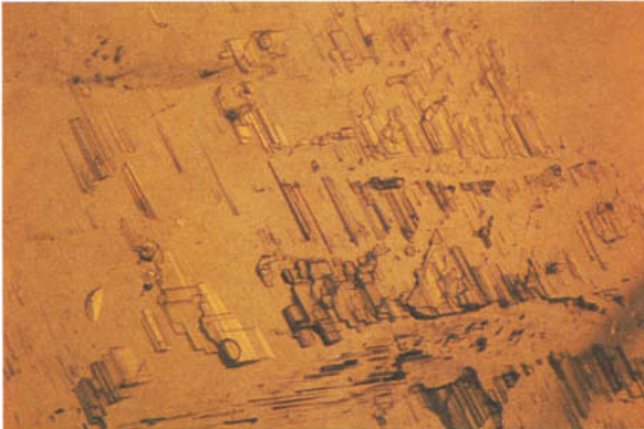
FIG. 2. A somewhat planar secondary partially healed fracture composed of numerous microscopic one- and two-phased inclusions. Transmitted light and shadowing. 110 \times .
