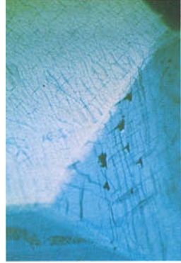
FIG. 11. Typical inclusion portrait of Lechleitner coated Type I synthetic emerald showing the 'net-like' cracks on the coating (see also Fig. 1). Transmitted illumination . Magnified 25x.
