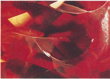
FIG. 22. Very fine cracks resulting in a Verneuil 'padparadschah' sapphire during the process of coating by Lechleitner. Dark-field illumination. Magnified 35× .
