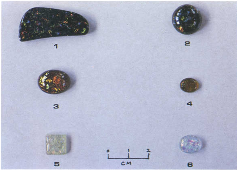
FIG. 1. Six Slocum Stones: 1 and 2, black opal simulants; 3 and 4, fire opal simulants; 5 and 6, white opal simulants.
