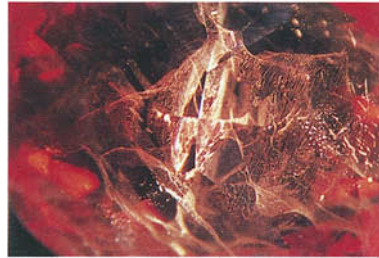
FIG. 21. 'Padparadschah' colour Verneuil synthetic sapphire experimentally coated by Lechleitner reveals fine fingerprint feathery structures, almost similar in appearance to those observed in Chatham synthetic orange sapphires. Dark-field illumination. Magnified 40× .
