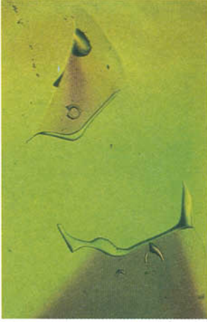
FIG. 8. Unusual bubble shapes associated with tinsel-like flakes. Fire opal simulant. 42x.
