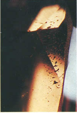
FIG. 17. The fingerprint cavities clearly exhibiting the dark fillings in synthetic yellow sapphire coated by Lechleitner. Transmitted illumination. Magnified 20x.
