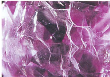
FIG. 24. All colours of Verneuil synthetic corundums are 'skinned' by Lechleitner — here a colour-changing type synthetic sapphire exhibiting many feathery structures internally after seeding technique. Dark-field illumination. Magnified 30× .
