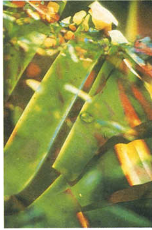
FIG. 6. Tinsel-like flakes showing spectacular interference colours separated by isotropic (black) glass. Fire opal simulant. Cross polarized light. 10X.
