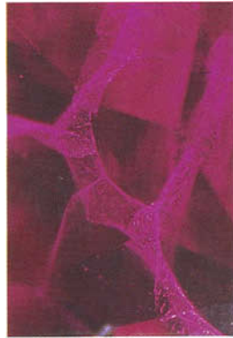
FIG. 18. Feathers resulting under high temperature in coated synthetic ruby appear almost similar to those seen in synthetic flux rubies. Dark-field illumination. Magnified 40x.
