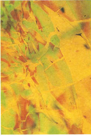
FIG. 4. Yellow, green and orange tinsel-like flakes. Fire opal simulant. 10X.
