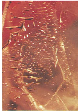
FIG. 14. A coated synthetic yellow sapphire with healed feather giving the stone a natural appearance. Dark-field illumination . Magnified 45x.
