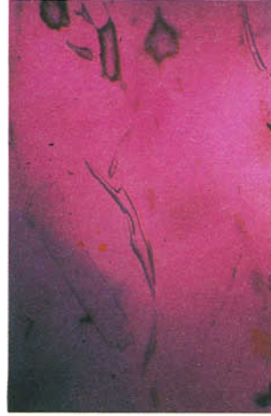
FIG. 14. High relief bubbles with spiky terminations. Black opal simulant. 42x.
