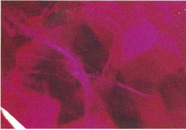
FIG. 20. Fine 'lace-like' feathers bunched in the central portion of a synthetic ruby 'skinned' by Lechleitner. Dark-field illumination. Magnified 38× .
