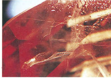
FIG. 23. Fingerprint feathers resembling those seen in natural 'padparadschahs' from Sri Lanka included within a coated Lechleitner corundum sample. Dark-field illumination. Magnified 20× .
