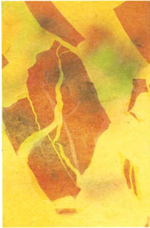
FIG. 5. Tinsel-like flakes with surface pattern resembling lunar cratering. Note the jig-saw like relationship between some of the flake margins. Fire opal simulant. 16X.
