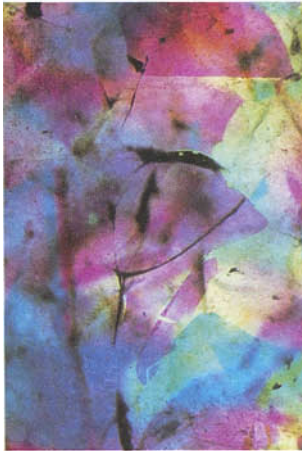
FIG. 3. Blue and purple tinsel-like flakes. White opal simulant. 10X.
