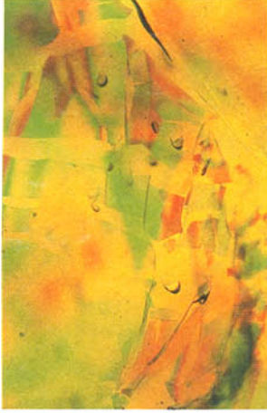
FIG. 10. High relief crescent-shaped bubbles and tinsel-like flakes. Fire opal simulant. 10x.
