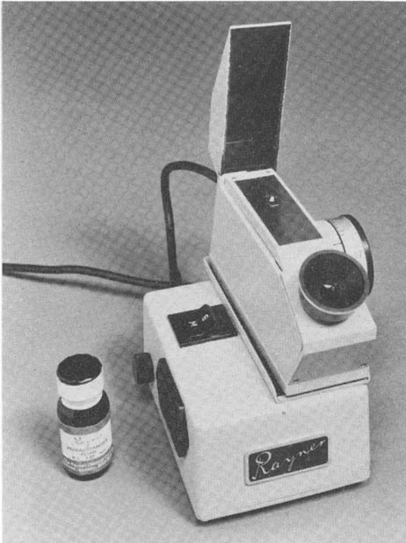
FIG. 5. The Rayner LED refractometer uses a 2-LED illuminator which can be withdrawn through the rear of the unit.
