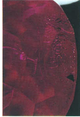
FIG. 15. The healed voids now containing a solid substance in a coated Lechleitner ruby. Dark-field illumination . Magnified 25x.
