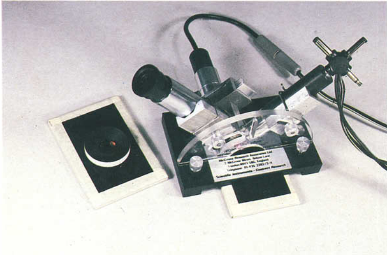
FIG. 6. The comparison prism spectroscope mounted on the basic spectroscope stand.
