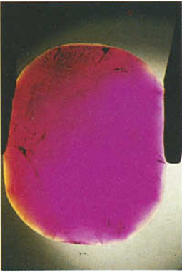
FIG. 8. A coated Lechleitner synthetic ruby seen in immersion microscope with diffused transmitted light . The colourless rim visible is the overgrowth. Magnified 20x.
