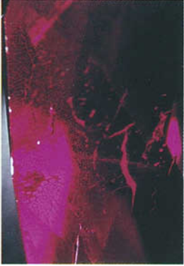
FIG. 13. Another ruby exhibiting the typical 'net-like' cracks on the coating. Dark-field illumination . Magnified 22x.
