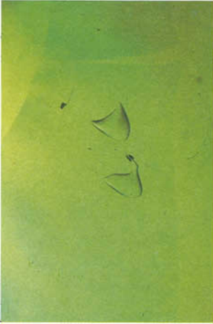
FIG. 12. Detail of two crescent-shaped bubbles. Fire opal simulant. 42x.
