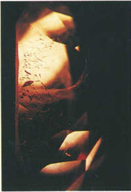
FIG. 16. Healed feathers, similar to those seen in Fig. 15, with included solid substance in a Lechleitner coated synthetic yellow sapphire. Transmitted illumination. Magnified 22x.
