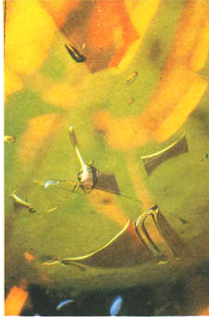
FIG. 9. Bizarre 'two-pronged' bubble (bottom right), elliptical bubbles and tinsel-like flakes. Fire opal simulant. 10x.
