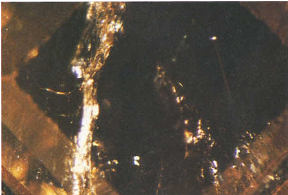
FIG. 3. Fracture system in a Canadian hessonite using partial immersion and darkfield illumination. 40 \times .
