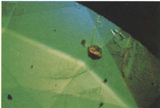
FIG. 7. Smoke-like veiling in Sri Lanka peridot. (40 \times ).
