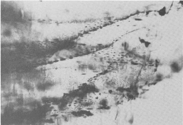
FIG. 10. Photomicrograph of a partly healed internal fracture ('feather', 'veil', or 'fingerprint') found in an aquamarine from O'Briens Creek. ( \times 25 magnification).
