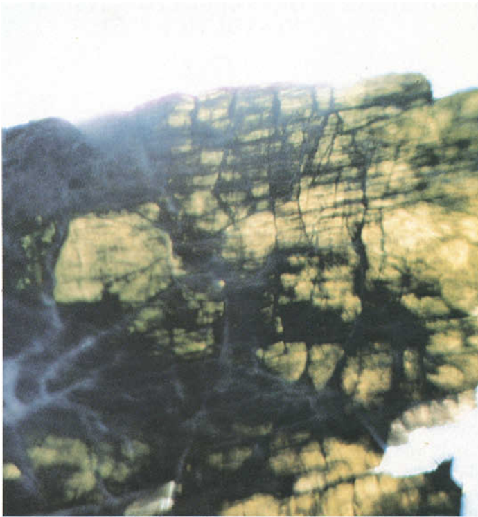
FIG.4. Thin section close-up showing nephrite translucency (3mm thickness: 3x magnification)
