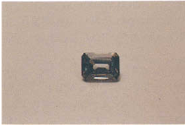
FIG. 8. A zircon weighing 2.10 ct in which the colour had altered from blue to a 'dirty colour' which was in parts brown and in other parts green.
