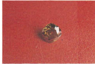
FIG. 5. A radium-treated green diamond weighing 2.66 ct (see Figures 4 & 6).
