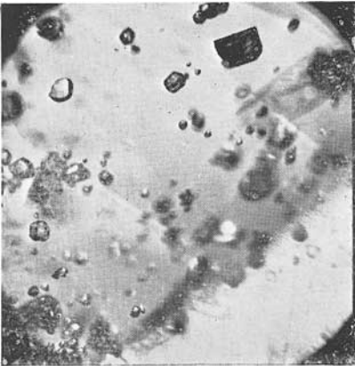
Fig. 3 — Inclusions in Ceylon Sapphires. 500 watt Nitrophot flood. \frac{1}{2} inch objective. 10 secs. exposure. Pan. roll film.
