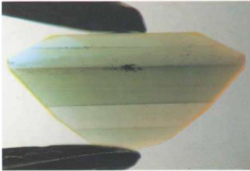
Fig. 3. Coloured growth bands in Seiko synthetic emerald, immersed in benzyl benzoate (length of stone, 4.94 mm).
