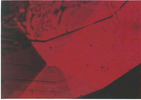
Fig. 11. Families of straight parallel growth planes that form angles, Chatham synthetic ruby; planes parallel to n ( 22\bar{4}3 ), r ( 10\bar{1}1 ) and n' ( 22\bar{4}3 ) form two angles of 154.0^\circ . - 35x.
