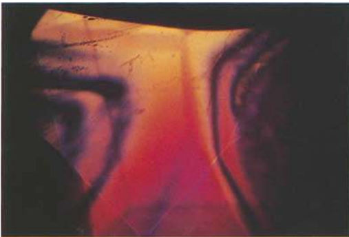
Fig. 24. Interference figure of a twinned natural amethyst, Uruguay; curved extinction bands. - x pol., 28x.
