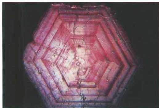
Fig. 9. Families of straight parallel growth planes that form an angle, Kenya ruby; planes parallel to prism faces a ( 11\bar{2}0 ) form an angle of 120^\circ . – 14x.
