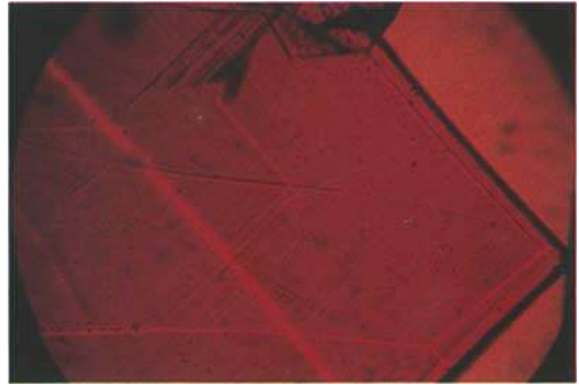
Fig. 15. Families of straight parallel growth planes that form an angle, Ramaura synthetic ruby; planes parallel to r and r' ( 10\bar{1}1 ) form an angle of 86.1^\circ . - 40x.
