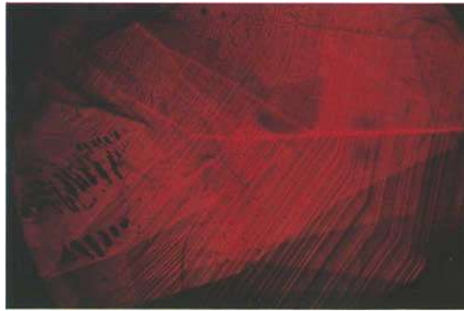
Fig. 13. Families of straight parallel growth planes that form an angle, Kashan synthetic ruby; planes parallel to r ( 10\bar{1}1 ) and n ( 22\bar{4}3 ) form an angle of 154.0^\circ . - 28x.
