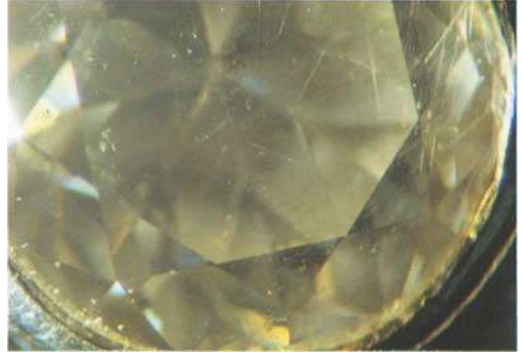
Fig. 6. Scratch marks seen in the plane of the girdle (junction plane) of the diamond-topped doublet depicted in Fig. 5.
