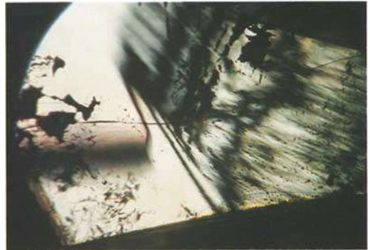
Fig. 30. Interference figure of a polysynthetically twinned natural amethyst, Bahia, Brazil; irregularly curved extinction bands. x pol., 30x.
