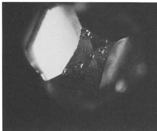
Orientated four-sided etch pits on the tetrahexahedral faces of the 0.21 ct 'star diamond' described.
