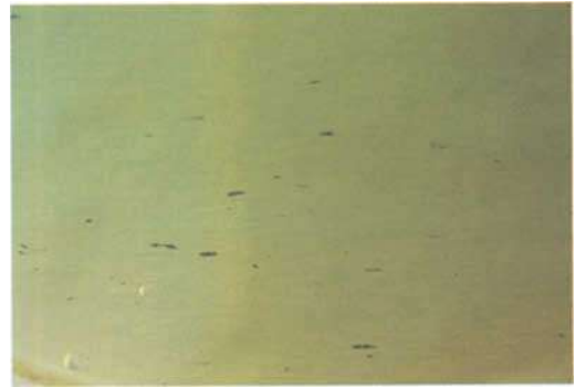
Fig. 4. Roughly rectangular inclusions of flux oriented in one direction within a Seiko synthetic emerald (approx. 60x magnification).
