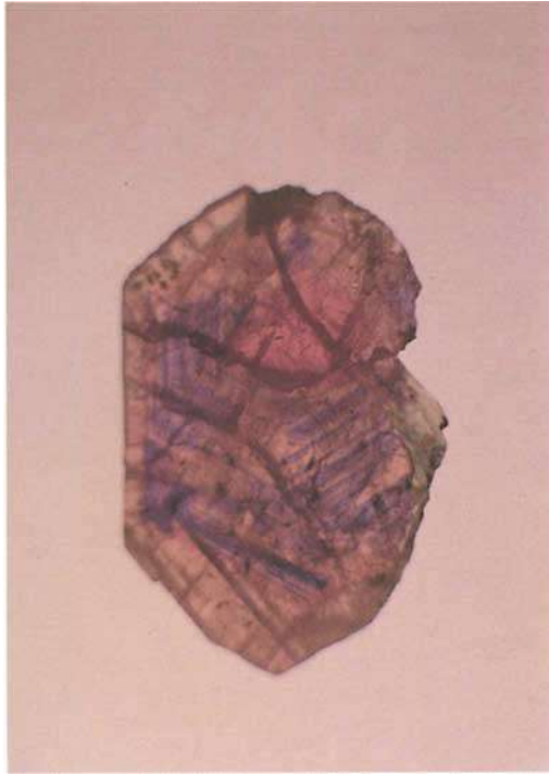
Fig. 6. Slice of ruby from the prismatic crystal showing colour zones, banding and inclusions.
