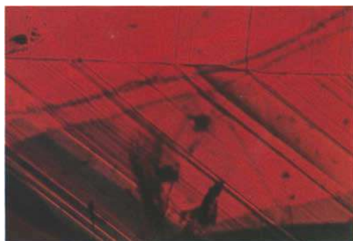
Fig. 10. Families of straight parallel growth planes that form an angle, ruby from Sri Lanka; planes parallel to prism faces a ( 11\bar{2}0 ) form an angle of 120^\circ . – 35x.
