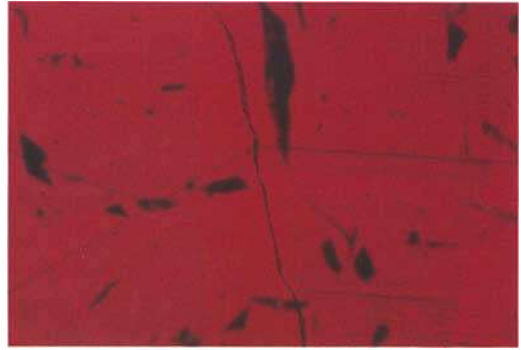
Fig. 12. Families of straight parallel growth planes that form an angle, Chatham synthetic ruby; planes parallel to d ( 01\bar{1}2 ) and n ( 22\bar{4}3 ) form an angle of 148.0^\circ . - 45x.
