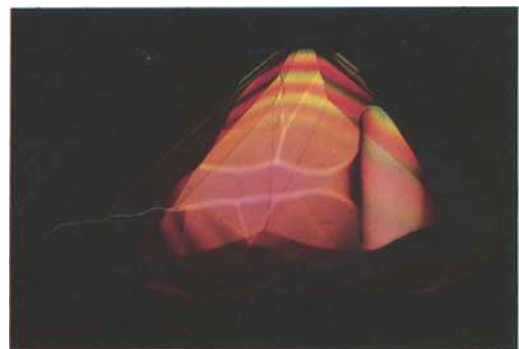
Fig. 19. Interference figure of an amethyst single crystal, the optic axis is nearly parallel to the table of the stone; synthetic amethyst of Russian production. - x pol., 20x.
