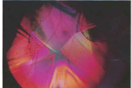
Fig. 23. Interference figure of a twinned natural amethyst, Zambia; twinning is observed only in sectors confined to the major rhombohedron and not in the sectors confined to the minor rhombohedron. - x pol., 20x.
